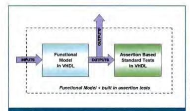
Figure 2: Extending model behaviour using assertions
