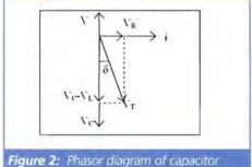
Figure 2: Phasor diagram of capacitor equivalent circuit
