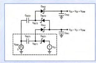
Figure 8: A voltage multiplier circuit based on basic bootstrap cell
