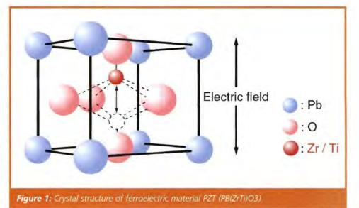
the ferroelectric crystals also changes. The process of polarisation itself is rapid, which leads to short writing times (~ 110ns). In addition, the energy required for polarisation, and hence the current consumption during saving, is extremely low. Integrated circuits read out the state of the electrical polarisation and recognise it as logical "1" or "0".
