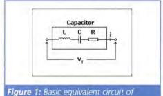
rigure 1: Basic equivalent circuit of capacitor
