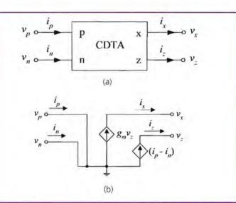
Figure 1: CDTA (a) circuit symbol (b) equivalent circuit
