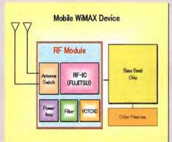
Block diagram of Fujitsu's WiMax IC solution
