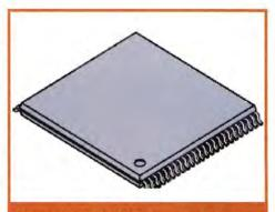
Figure 2: 2Mbit FRAM is currently the largest stand-alone FRAM memory from Fujitsu in mass production
