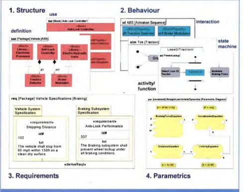
Figure 1: The four pillars of OMG SysML
