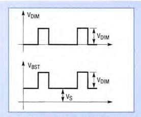
Figure 7b: Key waveforms of bootstrap circuit
