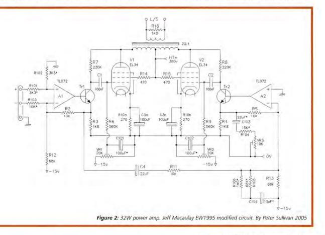
This will slightly affect the optimum setting of VR3 as it alters the emitter dynamic load impedance of Tr1.
