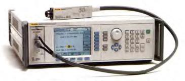
The Fluke 9640A comes with a 50 $\Omega$  levelling head and has an option to add a 75 $\Omega$  head, which extends the instrument's capability to calibrate workloads with 50 $\Omega$  and 75 $\Omega$  inputs
