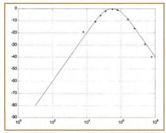
Figure 2: Calculated ( \_\_\_\_\_ ) and simulated ( \*\* ) bandpass filte
