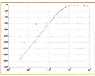
Figure 3: Calculated ( \_\_\_\_\_\_) and simulated ( \*\* ) highpass filter
