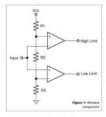
Resistors R1, R2 and R3 form a voltage divider, which generates the high and low threshold voltages. The outputs HIGH LIMIT and LOW LIMIT are both active high, generating a logic one on the HIGH LIMIT output when the input voltage rises above the high threshold, and a logic one on the LOW LIMIT output when the input voltage falls below the low threshold.
