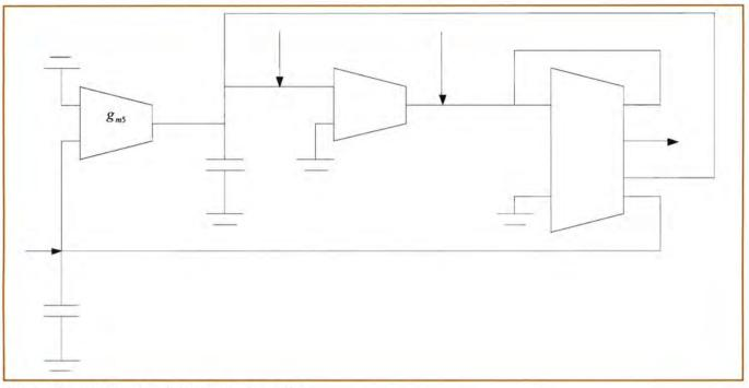
Figure 1: Proposed current-mode OTA-based universal filter
