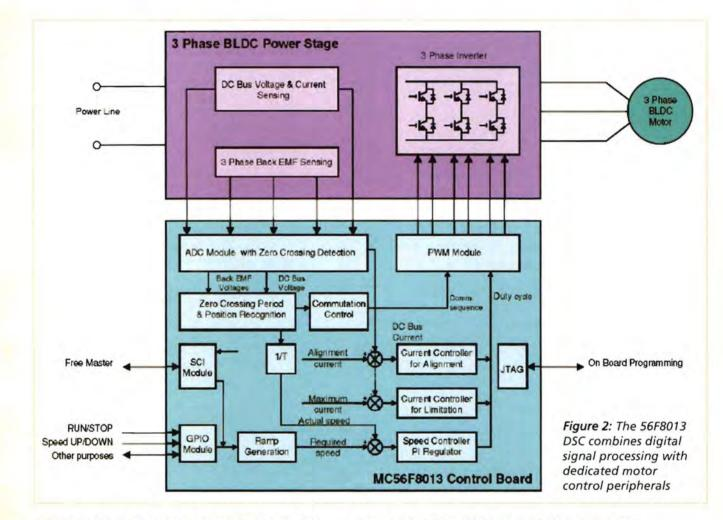
magnet rotor that produces the excitation magnetic field, with stator windings arranged in either two or three phases. In BLDC motors the windings are arranged so that each phase generates a trapezoidal magnetic field at the air gap along the stator. In the PMSM, the rotating field is sinusoidal.
