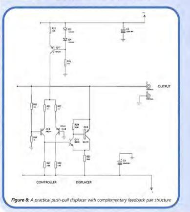
and distorted signal components. The reference is transferred by using the high-impedance output from transistor Q19 collector. Driver transistor Q15 is used to drive the Displacer Q14, so the control circuitry can work at low power levels.
