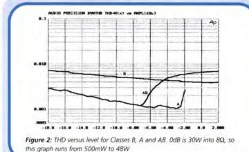
quiescent current of a Class-B stage. As this is done, an area of Class-A operation, with both output transistors conducting, is created around the zero-crossing. This can have very low THD indeed, at less than 0.0006% up to 10kHz, as demonstrated in one of my previous articles in
