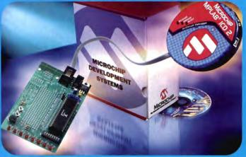
The MPLAB ICD 2 kit includes a demonstration board and samples of the PIC18F452 and PIC16F877 high-performance Flash micro-controllers. The demonstration board features a 2x16 LCD display, temperature sensor, EEPROM memory, LEDs, Piezo sounder, RS 232 interface. The kit also includes the MPLAB IDE (Interactive Development Environment) software.
