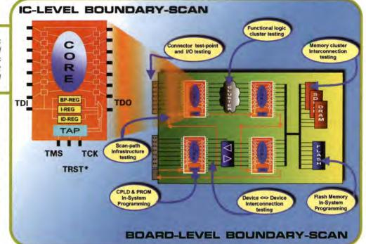
Figure 2: Boundary-scan as implemented within a device and how boundary-scan components can be daisy chained together at the board level
