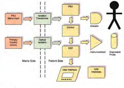
DSP device with lots of efficient processing power and the primary device can be a PIC or MSP430 style device. By carefully choosing the hardware around these devices, with as much of the safety critical monitoring done in hardware, it is possible in many cases to reduce the level of risk (level of concern).
