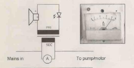
so a low voltage transformer is connected in reverse to increase the AC volts to 15V whilst current is flowing.
