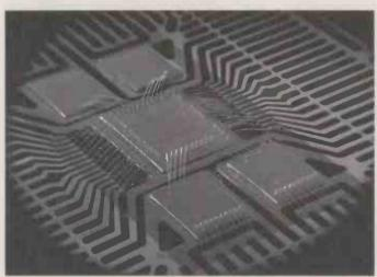
In this experimental automotive load driver a central load controller operates four power mosfets, offering smart protection during faults.
