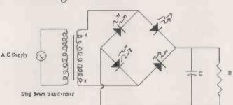
made of LEDs is connected to the output of a stepdown transformer and a load resistor is connected across the outputs. Rectification occurs as in an ordinary bridge but the ripple factor is found to be greater. In a bridge rectifier using ordinary
