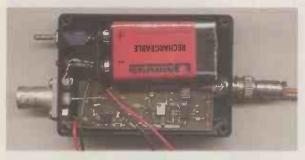
This uses the double balanced mixer/oscillator in the Philips SA612. The tuned components (L1 wound on a ¼ inch former; 6 turns) are set up for the 100MHz area, but can hopefully be scaled up to 200MHz. The 30pF tank capacitor can probably be replaced with a small trimmer if required, to extend the
