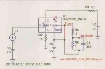
For DC set R4 to 0.001, V2 to 10v and V4 to 0v. For Transient set R4 to 0.1, V2 to 35v and V4 to 2.5v.
