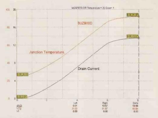
Figure 7: Used in self heating mode with an infinite heatsink at  $25\infty$ C ambient, this DC sweep of gate voltage from 0 to 8 volts with 10V drain-source, using the figure 1 circuit, shows how the junction temperature rise lags behind the power dissipated in the transistor, with increasing gate volts. Initially at room temperature, by the end of this sweep, junction temperature has risen to near 92°C.
