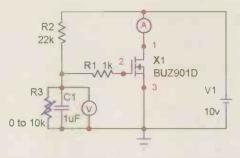
Figure 11: This simple test circuit allows direct measurement of drain current by gate voltage, for the critical subthreshold region that with three overlapping curves in the datasheet, was almost impossible to decipher.
