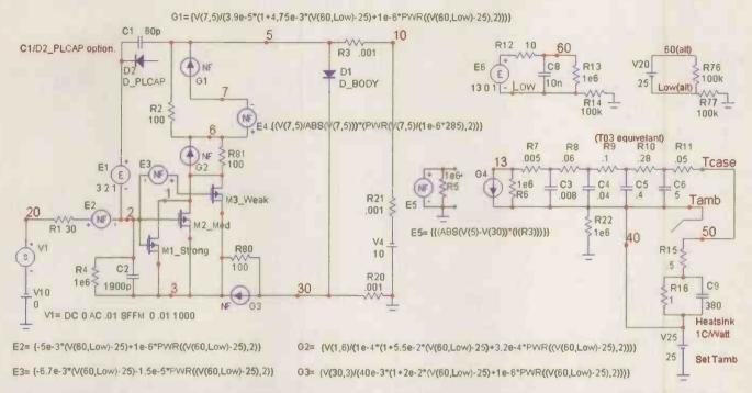
Figure 8: Having completed a model for the 'N' MosFet, the values used in the equations and the MosFet parameters were used to start the 'P' model development. However as can be seen in the figure, the polarity of a few components must be reversed and the three 'N' MosFet devices replaced with 'P' types. No changes are needed for the thermal control network.
