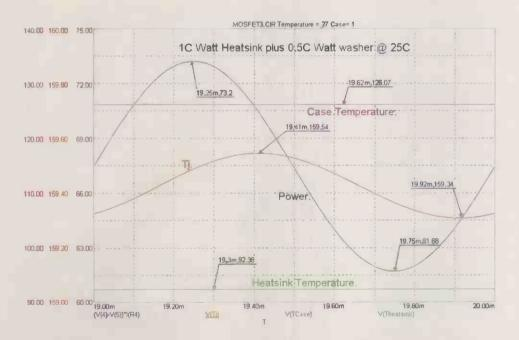
10) Removing the red link in figure 1 to now use the 1°C/watt heatsink and a mica washer, we see how dramatically the transistor junction and case temperatures increase. With much lower mean power dissipation of 67.5W, we see the junction temperature now exceeds the 150°C maximum rating for this device. The TO3 case temperature has risen to 126°C and the heatsink to a very hot 92°C.
