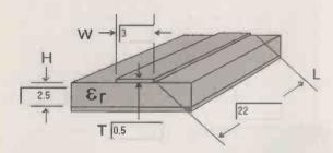
Figure 8: Layout of the obtained from radiation angle calculated using HP-AppCad  $\lambda/4$ transformation from 130 to 50Ω. The transformer is realised using a Teflon plate (22x30mm) and a copper stripe with W=3mm. Th=0.5mm, at the beginning of the Helix
