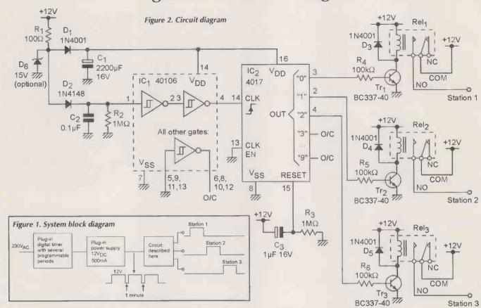
This simple circuit turns an ordinary mains timer into a multi-station controller for a garden sprinkler system. I had a spare timer and thought there must be a way to use it for automatic sprinkler control of more than one zone. This circuit might in general be a lower cost alternative to a commercial irrigation controller, since the latter costs a lot more than the common household timer.
