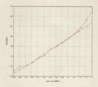
either way we need to remove at least 60dB of the fundamental in order to boost the system measurement capability by at least 60dB. The problem is that neither filter is testable on its own; they can only be tested as a pair. Figure 1: Measured second harmonic distortion characteristic of an Advantest R3261C spectrum analyser at 1.1MHz.
