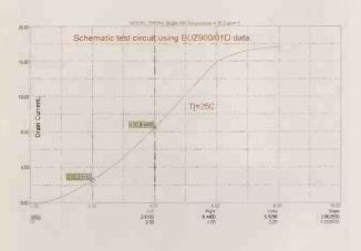
Figure 5: Attaining this smooth merging of the sub threshold conduction - square law regions, important when modelling distortion, completes stage 1 for our model. Our 25°C curve shows good agreement with the datasheet.
