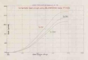
Figure 9: Using the final values for the 'N' device schematic model as starting values for the 'P' device schematic quickly produced these curves, closely replicating the datasheet subthreshold conduction, to complete our pair of schematic models.
