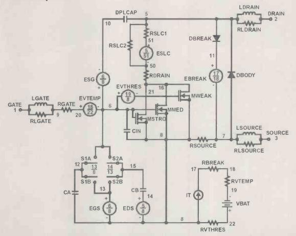
Figure 1: Fairchild's PSpice schematic for their FDP038 subcircuit model. Modelling audio frequency distortion, the circuit voltages used to drive the gate-source capacitance switches should not occur. To minimise convergence problems these switches were deleted from my audio models.
