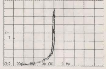
core transformer and the large current overshoot in fig. 4. The X-axis is related to current. The Y-axis is the phase shifted secondary voltage across the capacitor in fig.1.
