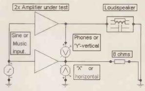
normally larger amplitude spiking would due to an amplifier's internal stability of NFB loop delayed current control in the presence of loudspeaker generated but phase shifted back EMF.
