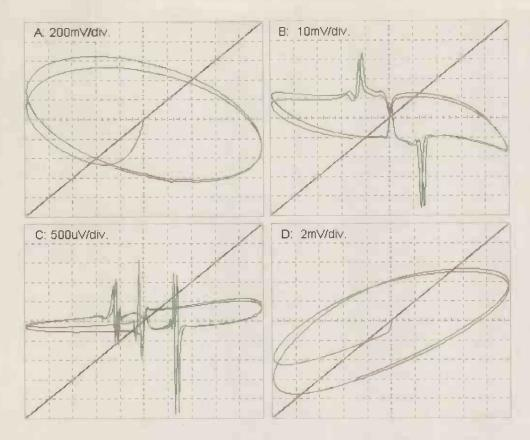
Figure 26: Four two-cycle 10V.RMS-10kHz 'live' interface distortion displays. phase shift with near resistive loss; i.e. the loudspeaker induced amplifier loss almost mirrors amplifier input. Note that even though this is an excellent sounding amplifier the error (not its output) potential is more shifted than steady sinewave plus resistor examination suggests!
