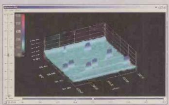
A 'waterfall' plot of a Bluetooth signal captured in real time by RFEL's SpectraChip MHz' prototype real-time spectrum analyser chip.
