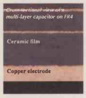
By using ceramics with "unstable surface characteristics", films can be created at room temperature, claimed Fujitsu.
