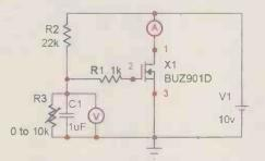
Figure 8: The simple test circuit used to measure the subthreshold region transfer curves, providing additional data points for this critical crossover region. Measuring a 'P' MosFet the supply polarity should be reversed.
