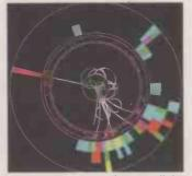
Simulated response of linear collider detector to supersymmetry displaying the characteristic signature of a lepton, a hadronic jet and missing transverse energy.
