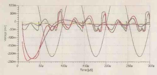
Figure 22: terminal residuals for the generic class-B, with and without its Miller connected VAS C.dom and output choke
