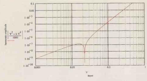
Figure 2: Theoretical second harmonic distortion due only to second and forth order terms in the power series representation.
