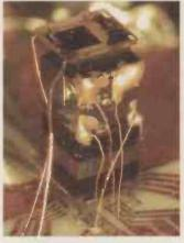
NIST has used a technique called coherent population trapping. A vertical laser diode is modulated at half the ground state frequency of caesium atoms in the cavity. Modulation produces sidebands that are separated by the caesium resonance frequency.
