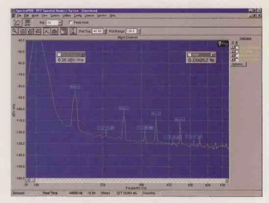
Fig. 6. Without diodes, but otherwise exactly as Figure 5, this Panasonic 'S'  $47\mu$ F 50 volt bi-polar aluminium electrolytic capacitor shows the distortion reduction available by changing a polar capacitor for a bi-polar type. With diodes, third harmonic increased more than 20dB to -99.24dB, further proof of the diode effect.
