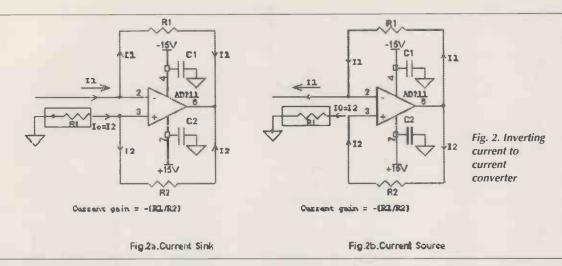
greater than the input current. The direction of the current that is delivered to the load is same as the direction of the input current.
