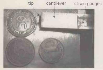
Fig. 8. The sample coins and the cantilever.
