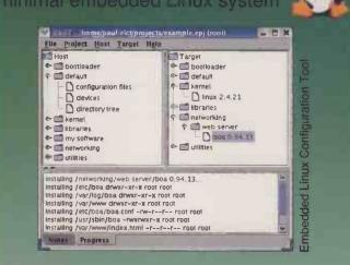
Select the software to include in your target project. Use ELCT to launch source configuration programs, compile source, check for library dependencies and install to the target.
