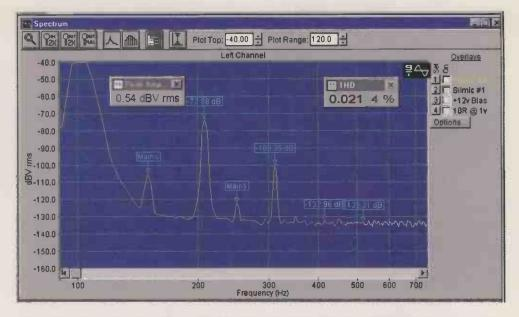
Fig. 2. Distortion results for a Silmic 100µF 25 volt rated polar aluminium electrolytic capacitor, with 12 volt DC bias and tested using  $10\Omega$  source impedance generating 1 volt across the capacitor. With no bias, second harmonic distortion for this capacitor was -93.2dB and -77.9dB with 6 volt bias.
