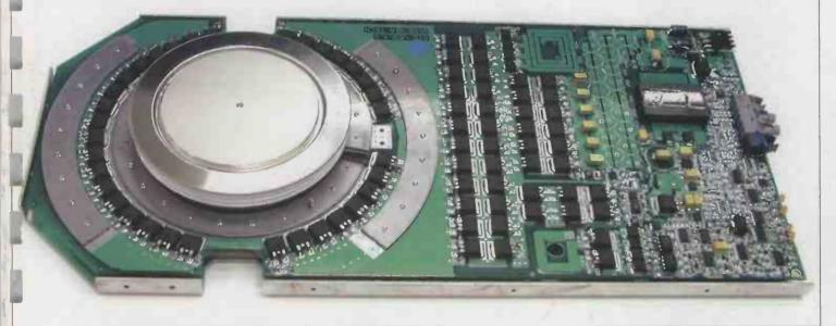
16 MW switch Accurate time measurement Project: Scanning force microscope
