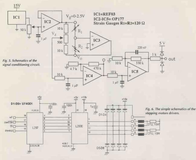
arm of the bridge is made of the two strain gauges  $(120\Omega)$ and the other one is made of two fixed resistors  $(10k\Omega)$ and a balancing potentiometer  $(500\Omega)$ , which allows zeroing of the system before starting scanning a sample.
