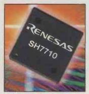
two on-chip Ethernet controllers that enable connection to two Ethernet LANs. Both peripherals make it suitable for security enabled devices for networks such as VPN dedicated boxes, home gateway servers, surveillance cameras and IP phones. The SH7710 is based on a SuperH Risc SH3-DSP CPU core that operates at up to 200MHz and achieves a processing capability of 260Mips. The on-chip DSP supports various kinds of
