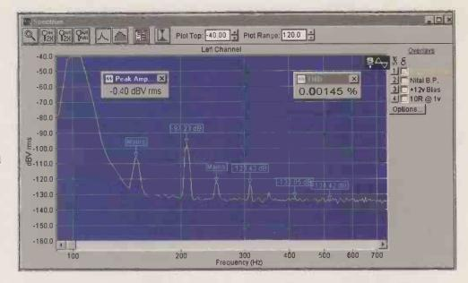
Fig. 9. Two 220µF 63 volt Nitai bi-polar capacitors in series made this 100µF "Double bi-polar" capacitor. Measured using a 1 volt AC and 12 volt DC bias as Figure 2, it generates almost twenty times less distortion. Second harmonic measured -101.75dB with 6 volt bias, -117dB unbiased.
