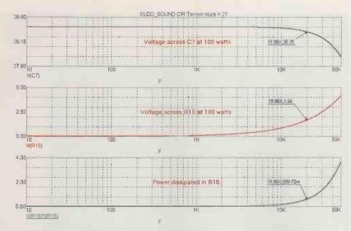
Fig.7. Using the Figure 3 simulation circuit to analyse for C7, we see the capacitor is highly stressed not resistor R15 and badly chosen C7 can generate large distortion. When an amplifier is used for high frequency sinewave tests with or without load, this capacitor frequently fails open, disabling the Zobel, the amplifier may oscillate. Yet R15 is frequently specified as 3 watt rating and C7 ignored.
