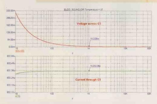
Fig. 4. One of eight simulations needed to accommodate C3 measured parameters by frequency, showing the 1kHz results. Voltage across C3 reduces with frequency but current through C3 remains almost constant regardless of frequency.
