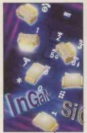
new devices are in the region of 35mcd at a forward current ( $I_F$ ) of 5mA. Maximum  $I_F$  is rated at 20mA, while each LED will handle a peak  $I_F$  of 100mA (pulse duration 30ms). Rohm
