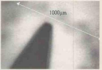
of chokes and lateral deflections of the cantilever when crossing sharp steps on the sample. Our device is affected by this problem because it does not have the feedback mechanism that allows SFM to work at constant force: in that case when the tip meets a sample relief, the sample holder is suitably displaced along z to keep constant the cantilever deflection.
