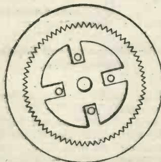
Fig. 3. — Showing how to attach a gear wheel to the underside of a condenser dial.
