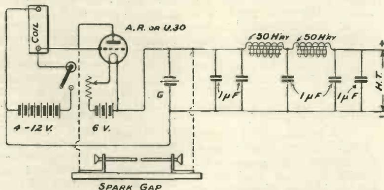
Fig. 1.—The connections of the complete supply circuit.
