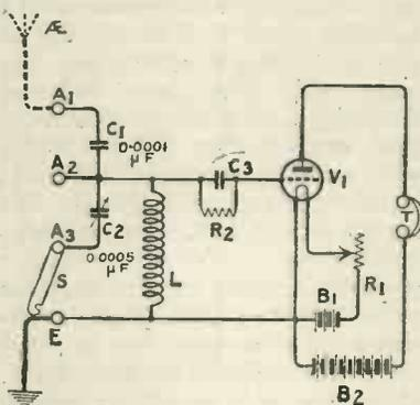
Fig. 2.—A four-terminal arrangement, permitting either series or parallel capacity.
