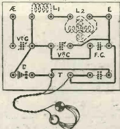
Fig. 4.—The wiring as seen through the panel.
