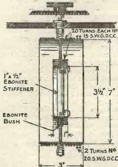
Fig. 3.—Details of the aerial tuning variometer.
