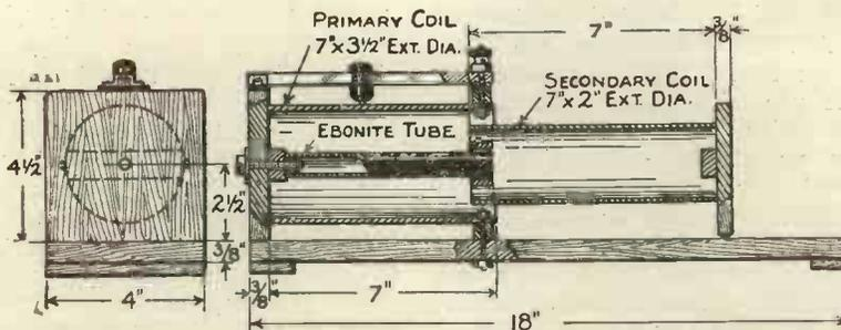
Fig. 2.—Details of the assembly of the parts.
