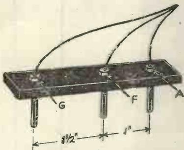
Fig. 6.—Details of the connecting lead for frame aerial use.
