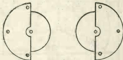
Fig. 1. — The necessary relative position of two panel-mounted condensers which are to be yoked.
