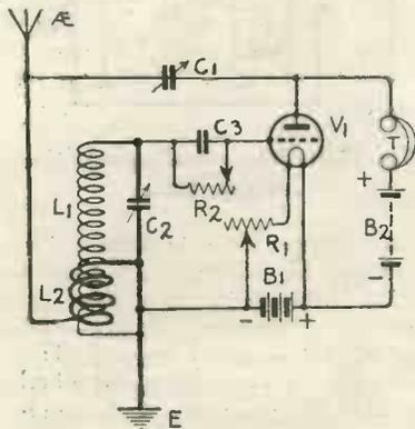
Fig. 14A.—An improved Reinartz Receiver.
