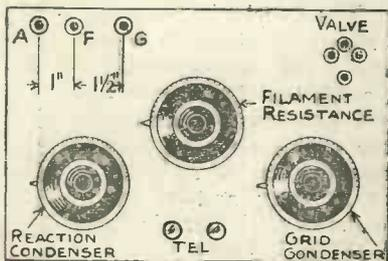
Fig. 7.—Plan view of the panel.
