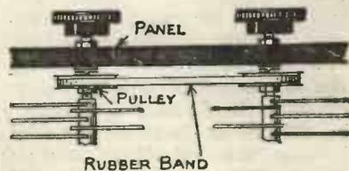
Fig. 2. — A simple and easy method of yoking condensers with two pulleys and a rubber band.
