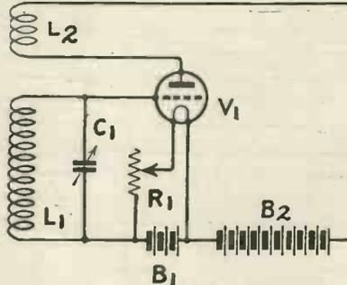
Fig. 1.—A simple oscillatory circuit.
