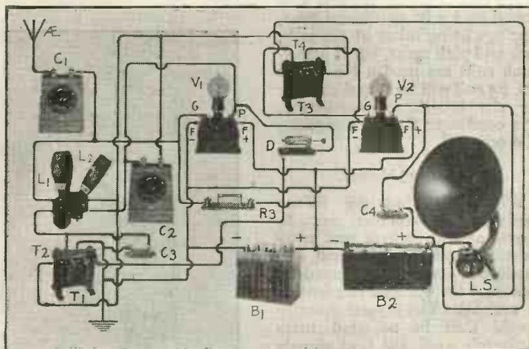
Fig. 20.—Pictorial form of the ST100 circuit.
