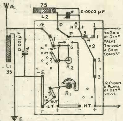
Fig. 16B.—The panel connections of Fig. 16A.
