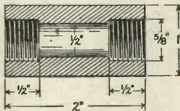
Fig. 1.—Details of the ebonite rod.
