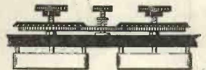
Fig. 5. — A method of coupling with gear wheels which is specially suited to mica condensers.
