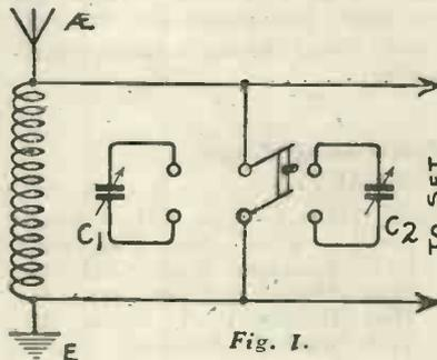
*Figs. 1, 2, 3, 4.—Illustrating the various methods of matching the condensers and anode coils.*
