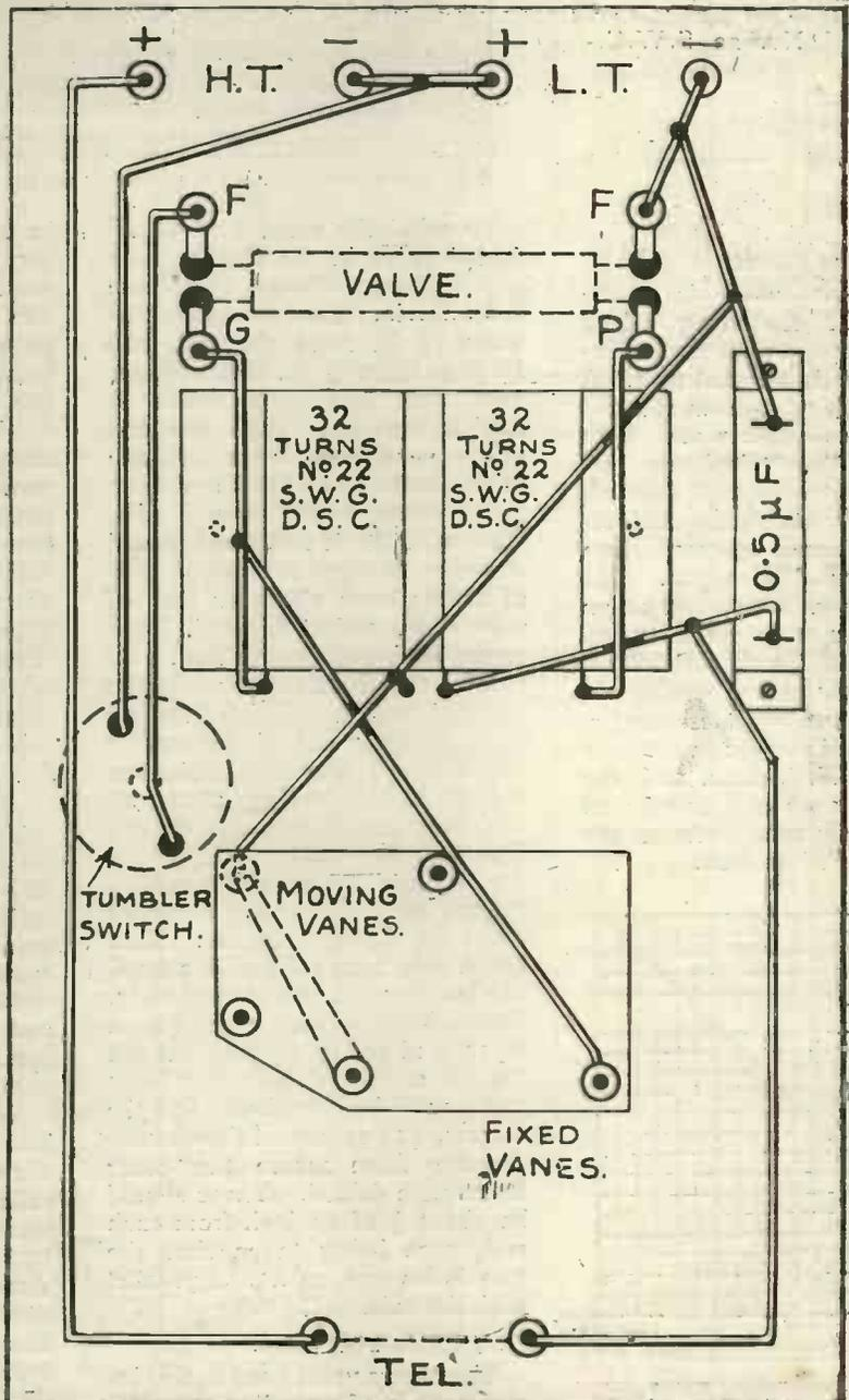
Practical wiring diagram. Points which are soldered are shown with a black dot. The connections to fixed and moving vanes are important.
