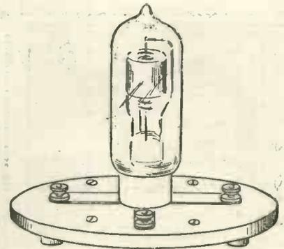
Fig. 3.—The valve mounted in position.
