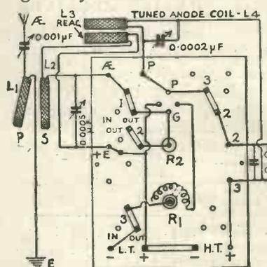
Fig. 20B.—The panel arrangements of Fig. 20A.
