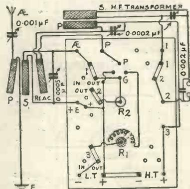
Fig. 19B.—The panel connections of Fig. 19A.
