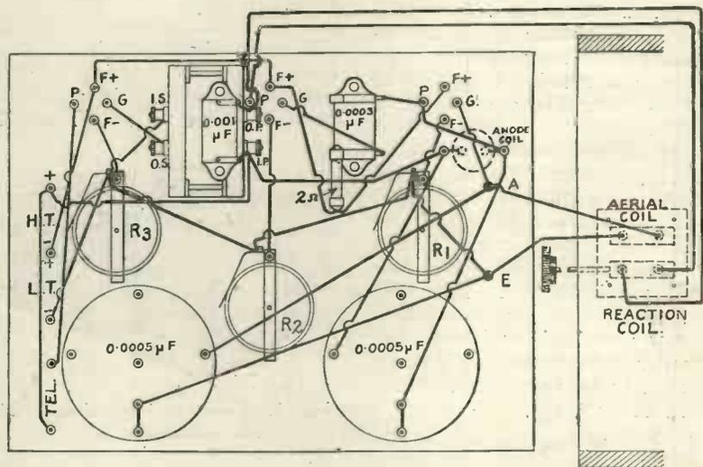
Fig. 6.—Wiring diagram of the receiver. A full-sized Blue-print of this drawing may be obtained from the offices of this journal, price 1/6.
