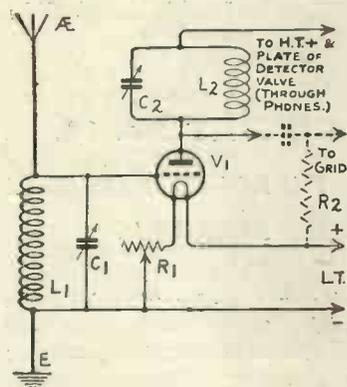
Fig. 16A.—A high-frequency tuned anode amplifier.
