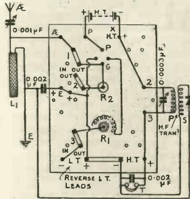
Fig. 21B.—The panel connections of Figure 21A.
