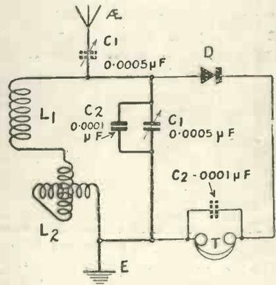
Fig. 7.—An example of a circuit which may be used with this receiver
