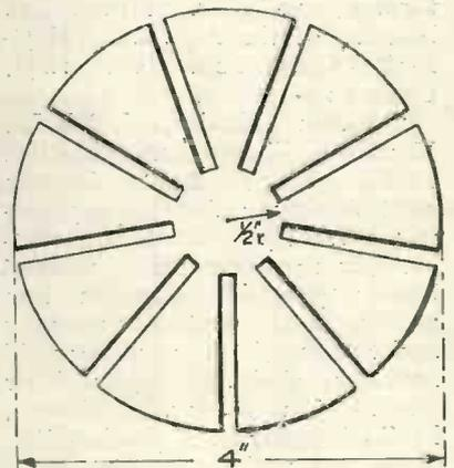
Fig. 3.—Dimensions for a disc type former.
