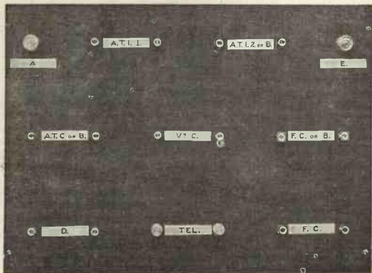
Fig. 8.—The top of the panel, showing the position of the various plug-in components.
