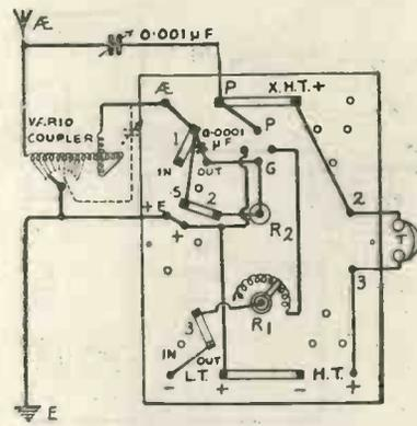
Fig. 13B.—The panel connections of Fig. 13A.
