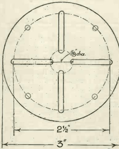
Fig. 2.—Constructional details of the adaptor.
