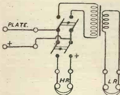
Fig. 3.—Circuit arrangement for using both H.R. and L.R. 'phones.
