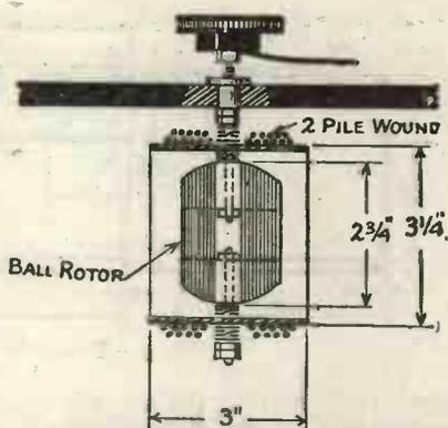
50 TURNS NO. 20 S.W.G. D.C.C. ON STATOR ROTOR FULL OF SAME. REACTION—40 TURNS NO. 22 S.W.G. D.C.C. ON STATOR. ROTOR FULL OF SAME.
