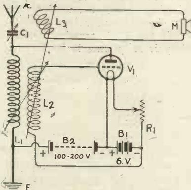
Fig. 22A.—A simple single valve transmitter circuit.
