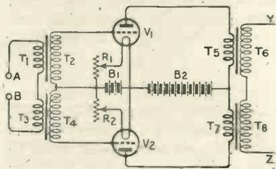
Fig. 1.—The "push-pull" amplifier circuit.
