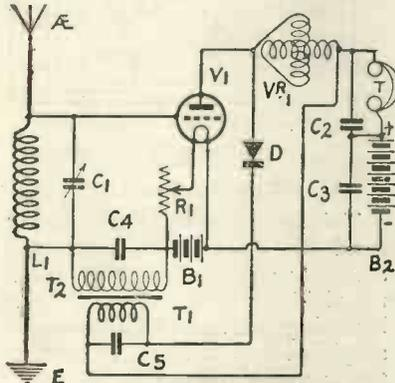
Fig. 11A.—A Reflex Receiver with Variometer Tuned Anode.
