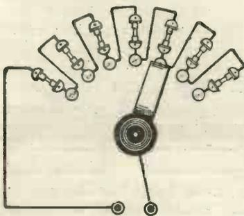
Fig. 1.—How the variation of resistance is obtained.
