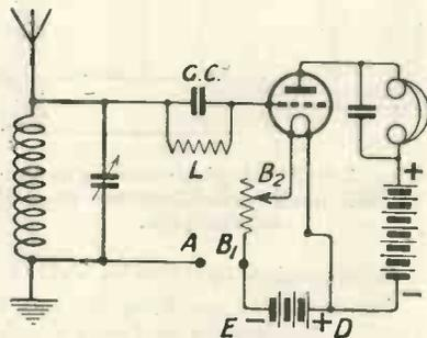
Fig. 1.—A simple valve detector circuit without reaction.
