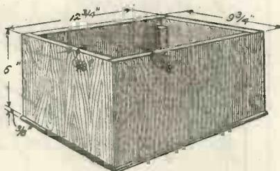
Fig. 5.—Constructional details of the containing box.
