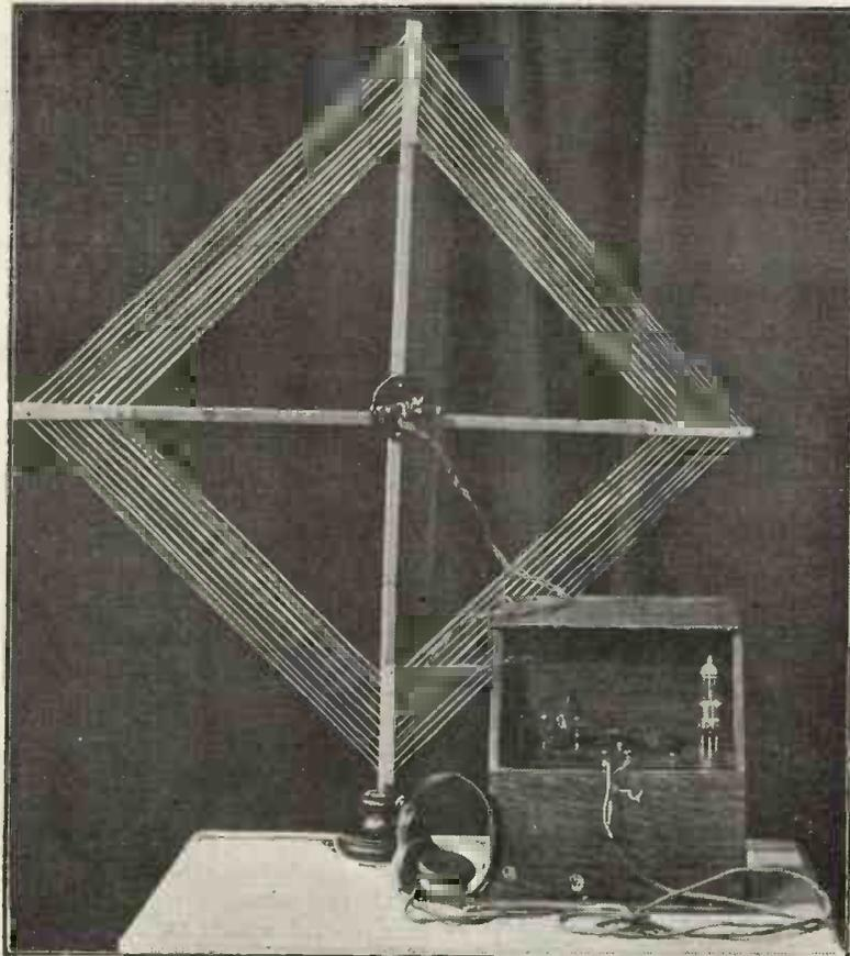
Fig. 1.—The receiver connected to the frame aerial.
