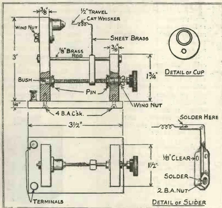
Constructional details of the detector.
