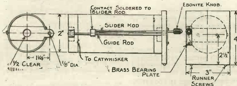
Fig. 3.—How the secondary is assembled.
