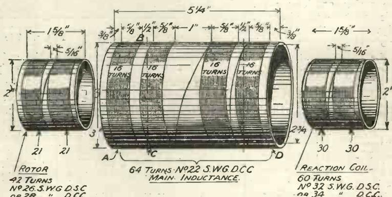
Fig. 4. Constructional details of the Tuning and Reaction Coils.
