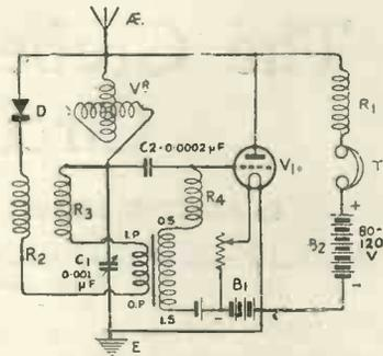
Fig. 3.—The circuit with the addition of a low-frequency transformer to give reflex amplification.
