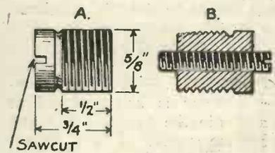
Fig. 2.—Dimensions of brass plug.
