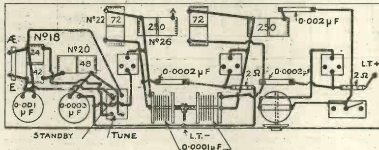
Fig. 4.—The H.F. Wiring.
