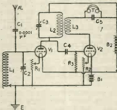
Fig. 1.—The ST34 circuit arranged for constant aerial tuning.
