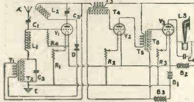
Fig. 31.—The ST118 Circuit.
