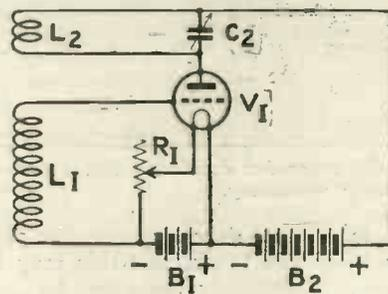
Fig. 2.—A self-oscillating arrangement in which the anode circuit is tuned.
