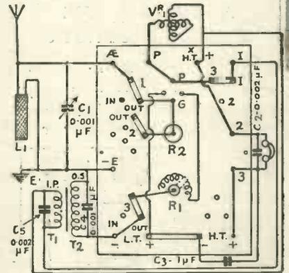
Fig. 11B.—The panel connections of Figure 11A.
