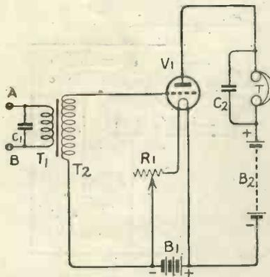
Fig. 15A.—A low frequency amplifier circuit.
