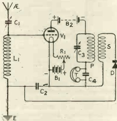
Fig. 21A.—The Voigt dual amplification circuit.
