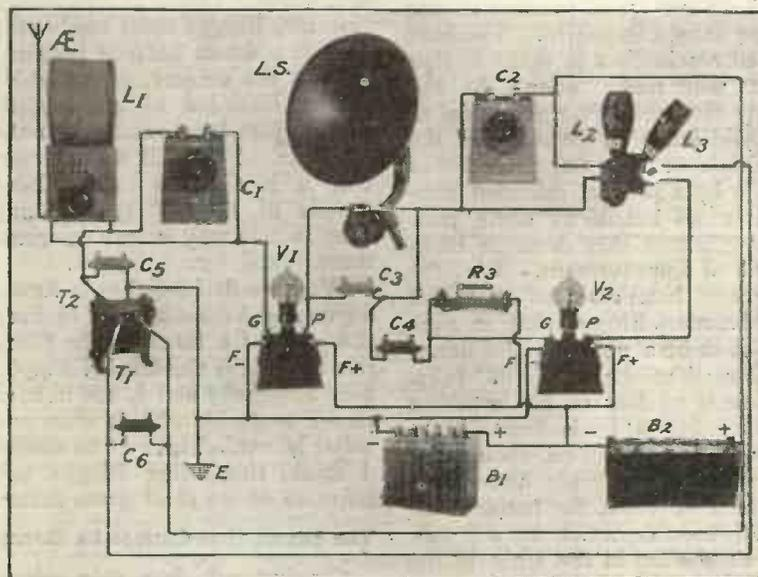
Fig. 28.—Pictorial form of the ST75 Circuit.
