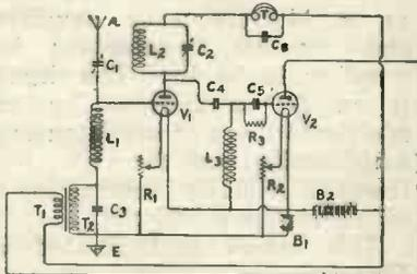
Fig. 29.—A special dual circuit.
