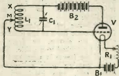
Fig. 4.—A self-oscillating system employing a single circuit.
