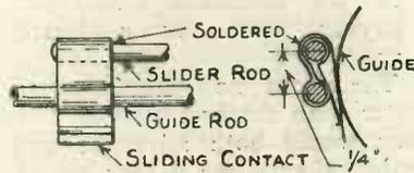
Fig. 4.—Details of the slider.
