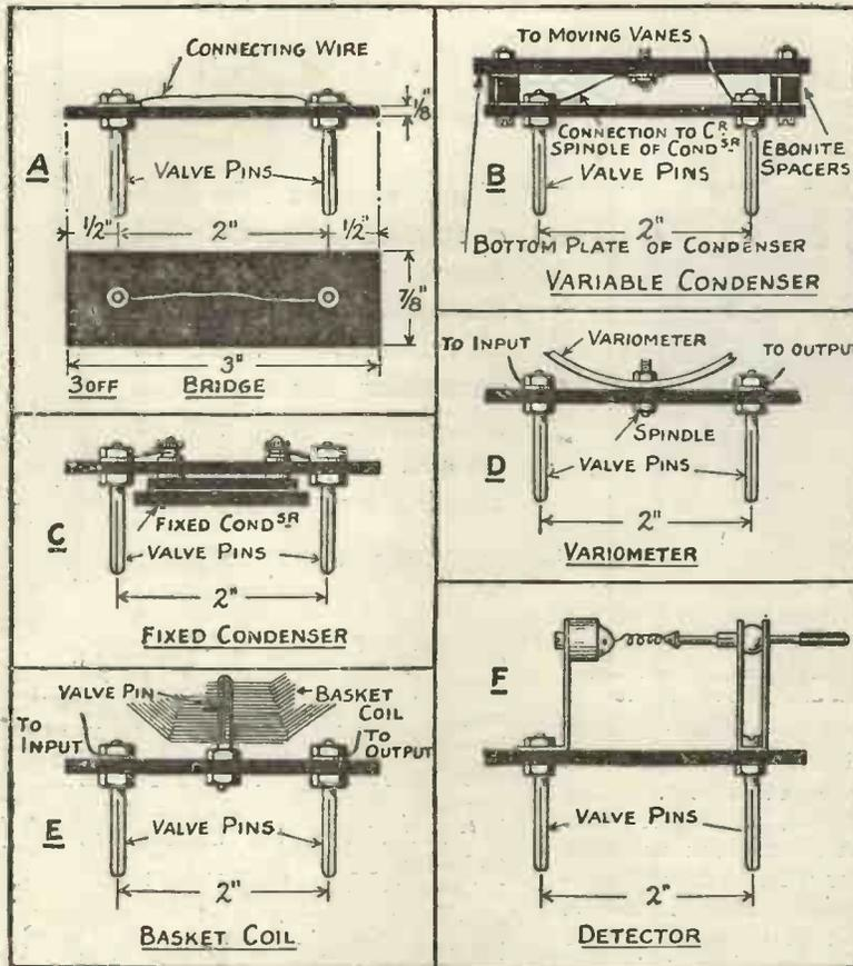
Fig. 5.—Illustrating the different plug-in units.
