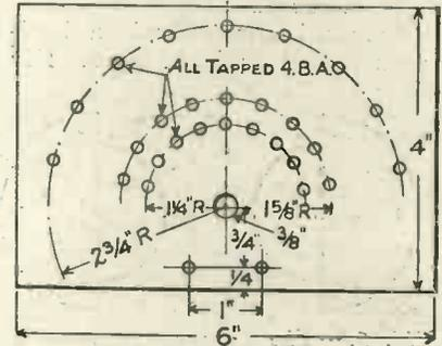
Fig. 3.—Drilling plan of the switch.
