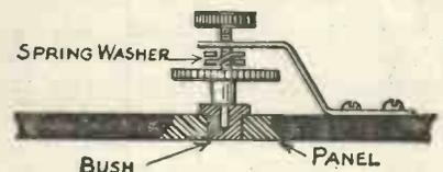
Fig. 4. — Details of the operating knob and gear wheel for the scheme shown in fig. 5.
