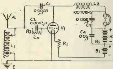
Fig. 5.—The circuit of the receiver. Note the use of the 100-turn coil L2.
