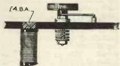
Fig. 2. The constructional details of the switch and resistance.
