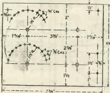
Fig. 4.—Drilling plan of the front panel.
