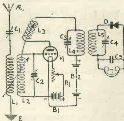
Fig. 19A.—A single-valve-crystal reaction receiver.
