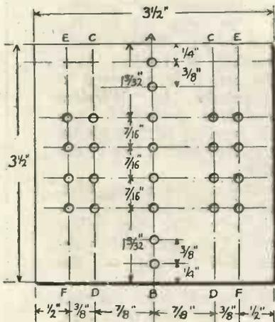
Fig. 2.—Constructional details of panel.
