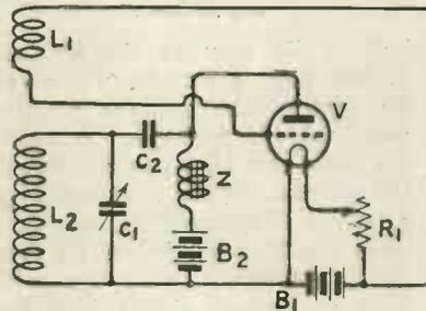
Fig. 3.—Use of iron or air-core choke.
