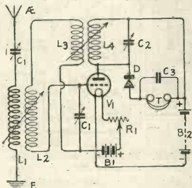
Fig. 20A.—A valve-crystal regenerative circuit.
