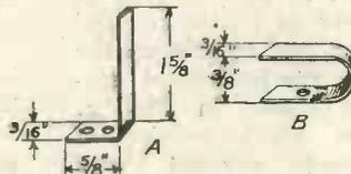
Fig. 3.—Details of the two types of contacts.
