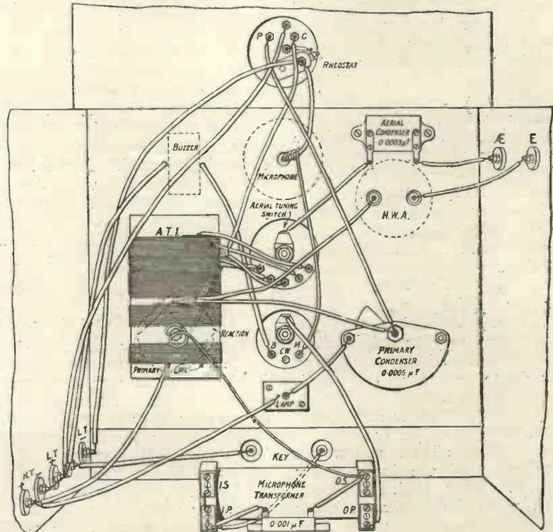
Fig. 8.—Complete wiring diagram of the Transmitter.
