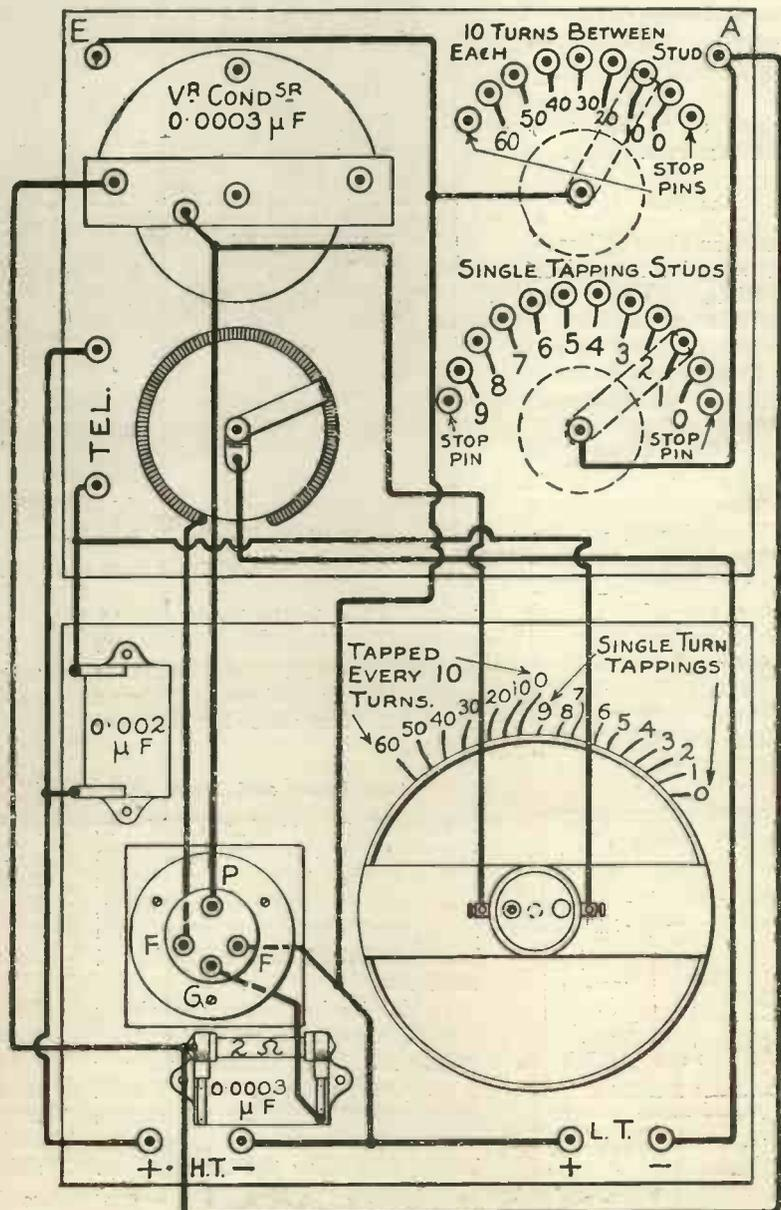
Fig. 7.—Complete wiring diagram.
