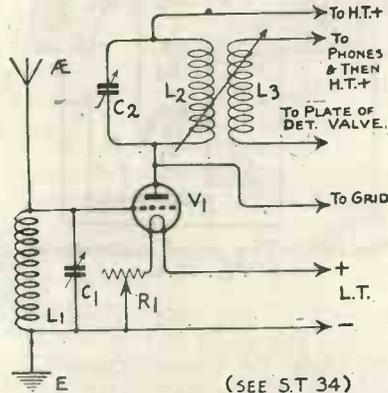
Fig. 17A.—H.F. amplification with tuned anode reaction.
