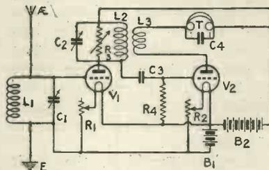
Fig. 1.—Controlling reaction with a damping resistance.
