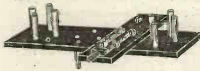
Fig. 1.—The double valve holder.
