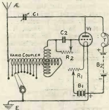
Fig. 13A.—A modified Reinartz Receiver.
