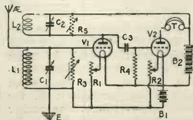
Fig. 2.—Showing how a damping resistance may be connected when reaction upon the aerial is used.
