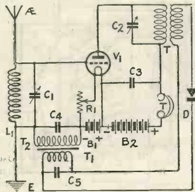
Fig. 10A.—A Reflex Receiver with Transformer.
