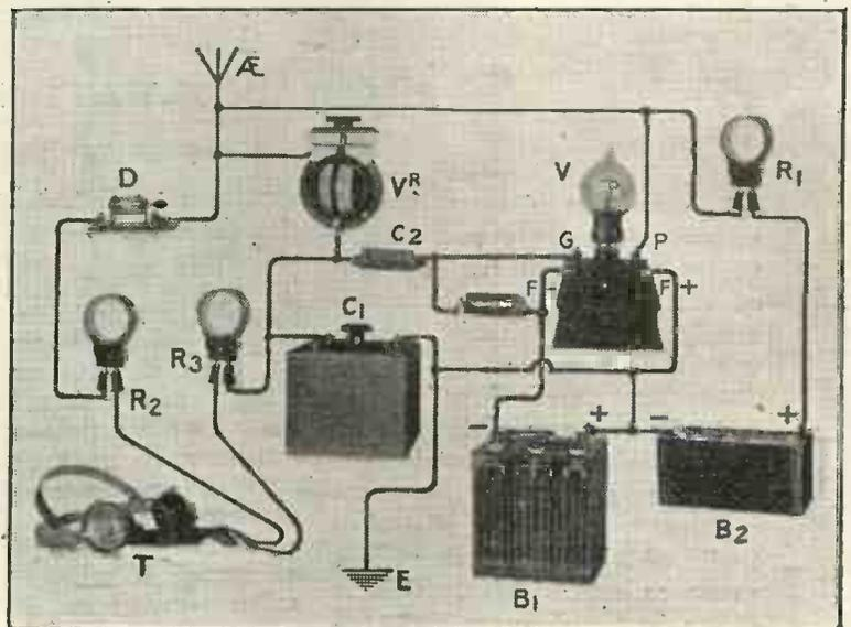
Fig. 2.—The circuit of fig. 1 shown pictorially. The coils R1, R2, and R3 are the radio chokes, and may be ordinary plug-in coils.
