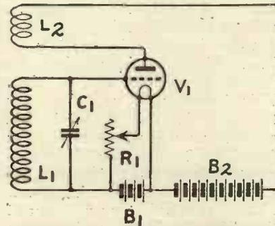
Fig. 1. A simple circuit for the production of oscillations.
