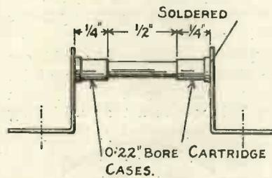
Fig. 2.—Dimensions and details of the resistances.
