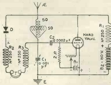
Fig. 1.—A single H.F. amplifying circuit employing the Ultraudion principle.
