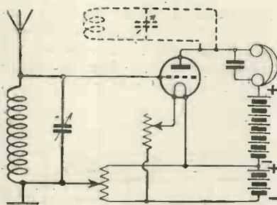
Fig. 2.—A single valve detector circuit with potentiometer control of the grid.
