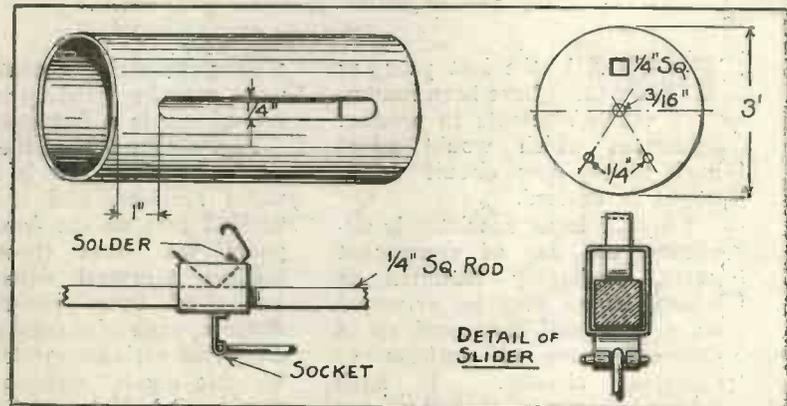
Figs. 1, 2, 3 and 4, showing constructional details of the secondary coil and slider.
