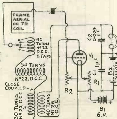
Fig. 18A.—A single valve super-regenerative circuit.
