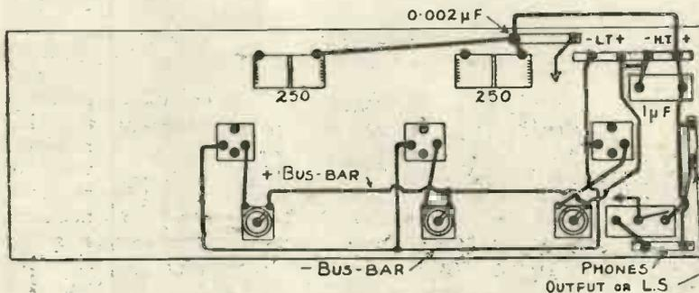
Fig. 3.—The L.T. and H.T. Wiring.
