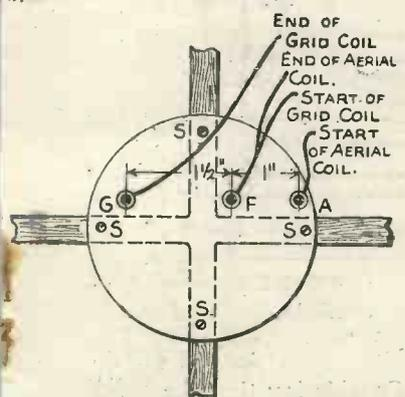
Fig. 5.—Illustrating how the ends of the coil are connected to the valve legs
