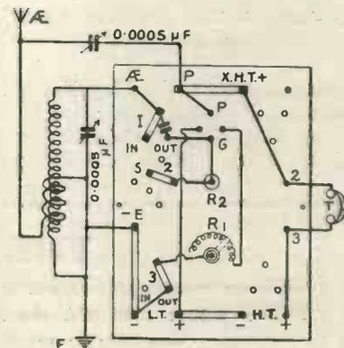
Fig. 14B.—The panel connections of Fig. 14A.
