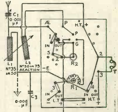
Fig. 12B.—The panel connections of Figure 12A.
