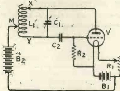
Fig. 5.—A rearranged circuit using a grid leak.
