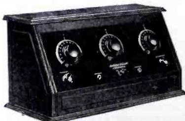
two stages of tuned radio-frequency amplification, detector and two stages of audio amplification.
