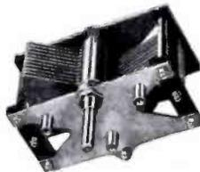
No. 301-A Low-Loss Condenser. Grounded rotor type with straight line curve. Capacity range .00009 to .0005. Ideal for use in conjunction with No. 105 and No. 205 coils.
