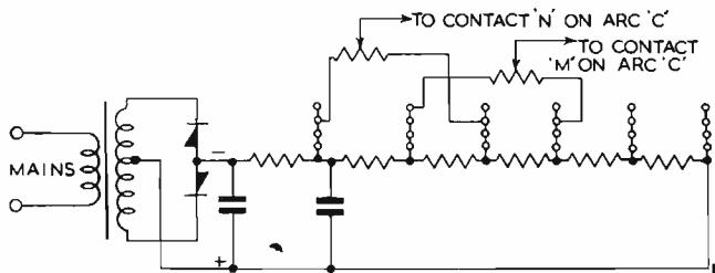
Fig. 2. Source of comparison voltage
