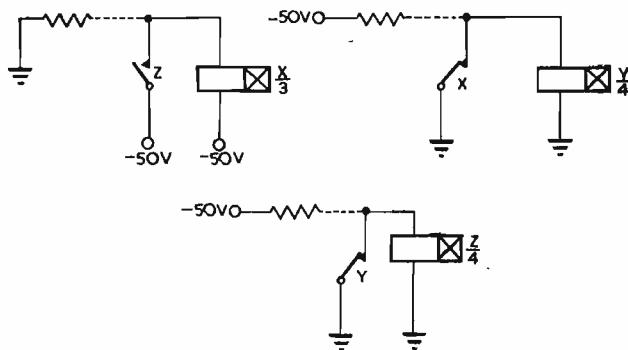
Fig. 3. Timing relays
