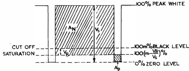
Fig. 15. Assumed operating conditions of a double limiter when designed for maximum rejection of noise modulation
