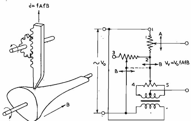
Fig. 10. Three-dimensional cam
