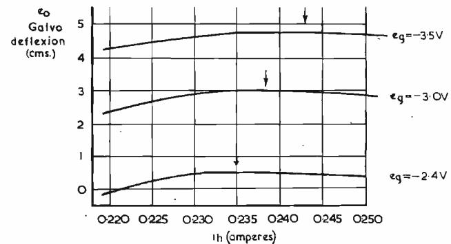
Fig. 5. Barth circuit—variation of balance point with control grid potential
