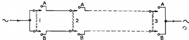
Fig. 1. Conventional two-position interlock (two switch poles used). Circuit is made only with "all A's" or "all B's."
