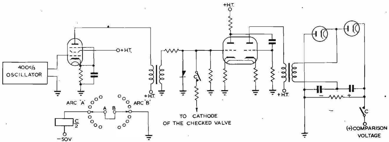
Fig. 8. Measurement of a low D.C. potential
