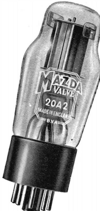
**IMPORTANT:** Cathode and Heater should normally be tied externally. If left free the Heater to Cathode Voltage must never exceed 25 volts peak. The heater must be switched on for 15 seconds before anode voltage is applied.
