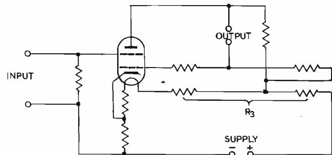
Fig. 1. Dubridge and Brown circuit, with input resistor for current measurement by direct deflection method
