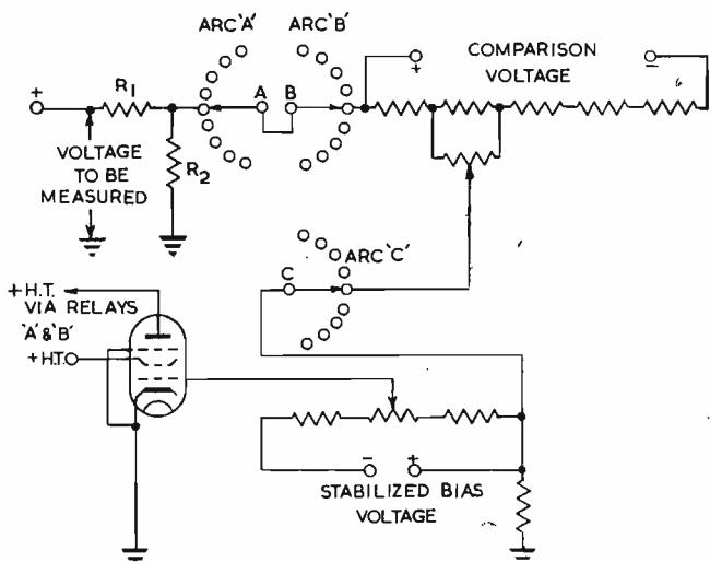
Fig. 6. Measurement of a high D.C. potential
