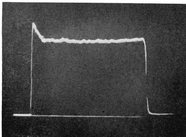
load conditions is shown in Fig. 2. The arc voltage is represented by the height of the oscillograph deflection above the base line. This height may, of course, be measured by applying a variable known sinusoidal voltage to the input of the amplifier and drawing a calibration curve of the whole apparatus.
