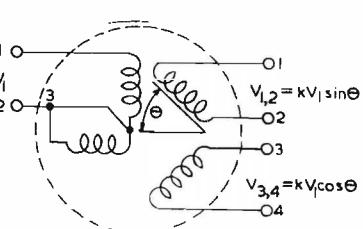
Fig. 5. Resolver No. 1. Resolution of polars to cartesians
