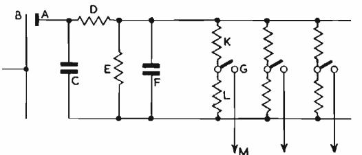
Fig. 4. Circuit of electrical network for different polarizing voltages
