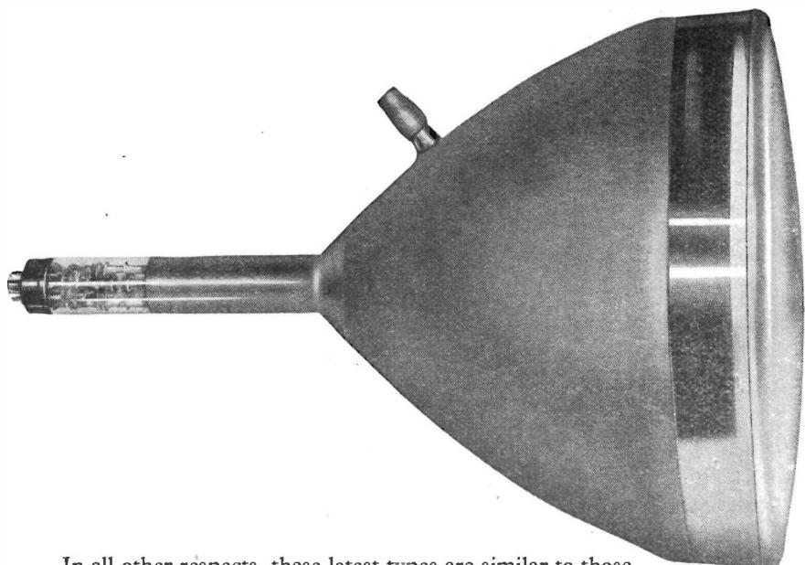
In all other respects, these latest types are similar to those they replace: aluminised screen for longer life and outstanding brilliance; external conductive coating, which, in conjunction with the internal coating, can be used as the E.H.T. reservoir capacitor; and the standard international octal base.
