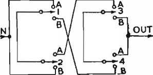
Fig. 4. Interlocking of four switches
