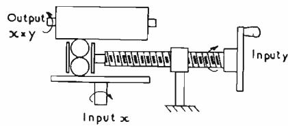
Fig. 2. Mechanical multiplication
