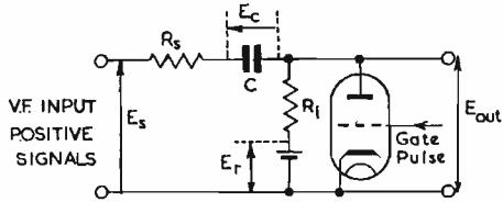
Fig. 16. Black level restoration circuit
