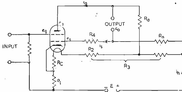
Fig. 2. Barth circuit with input resistor for current measurement by direct deflection method
