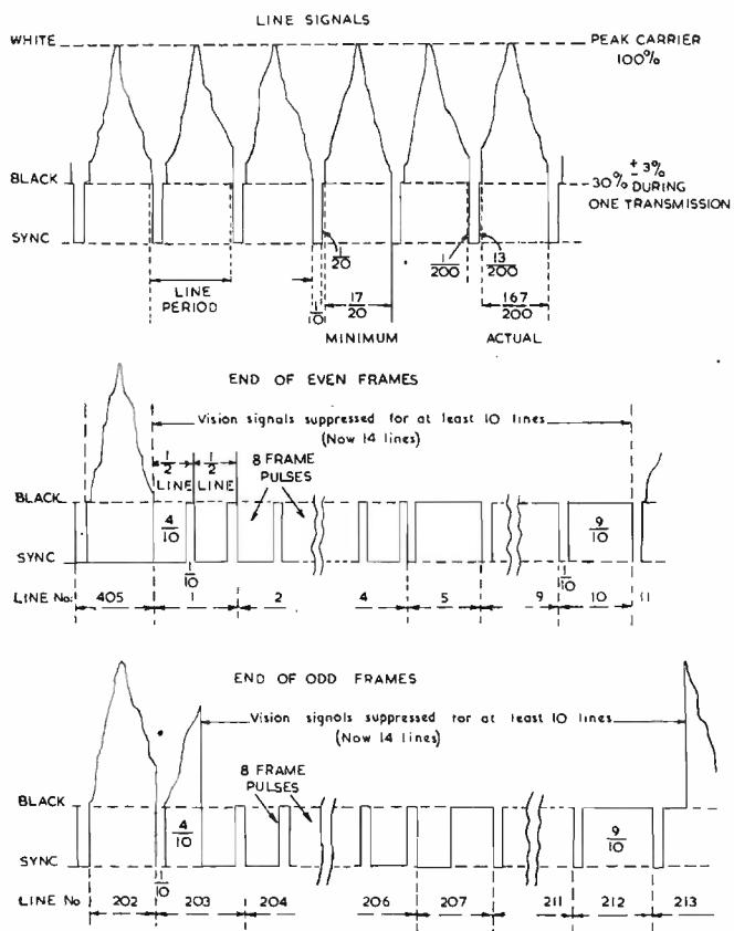
Fig. 19. Vision waveforms
