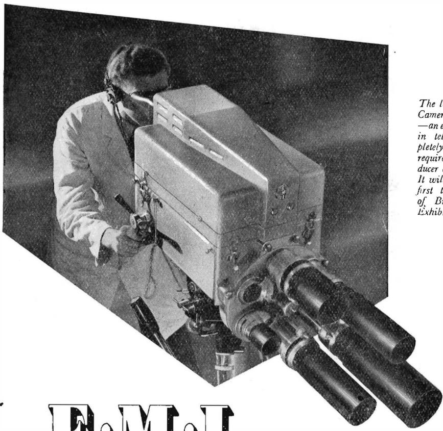
*The latest C.P.S. Emitron Camera with 6 lens turret—an entirely new conception in television which completely satisfies the exacting requirements of both producer and operator.*
