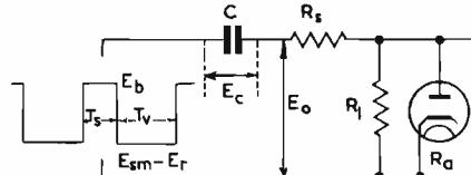
Fig. 17. Equivalent circuit of Fig. 16 referred to in the text
