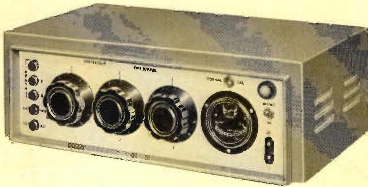
One milliwatt output on 600 ohm line (.775 V) for an input of 30 microvolts on 7.5—30 ohm balanced input. Output balanced or unbalanced by internal switch. The meter reading is obtained by a valve voltmeter with 1 second time constant, which reads programme level, and responds to transient peaks.
