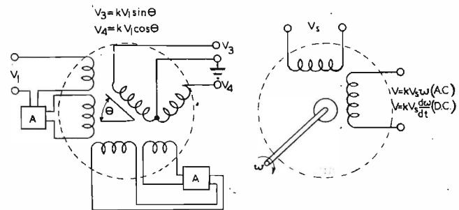
Fig. 6. Resolver No. 2. Resolution of polars to cartesians
