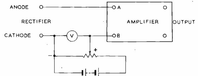
Fig. 3. Connexions for arc voltage measurement
