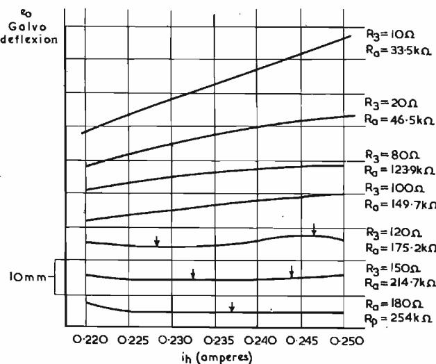
Fig. 7. Caldwell circuit—determination of minimum value of  $R_3$  necessary for balance (the vertical separation of the curves is arbitrary)
