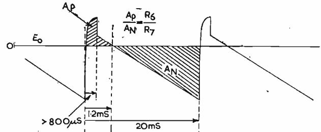
Fig. 23. Equivalent waveform  $E_o$  obtained when the anode waveform of a short flyback frame time base is passed onto the clamp valve grid via a resistance ratio  $R6 : R7$  of Fig. 20
