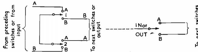
Fig. 2(a). Basic arrangement of two switches (single pole switches used)
