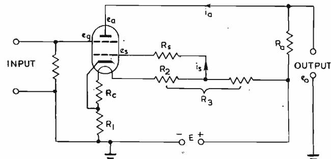
Fig. 3. Caldwell circuit with input resistor for current measurement by direct deflection method
