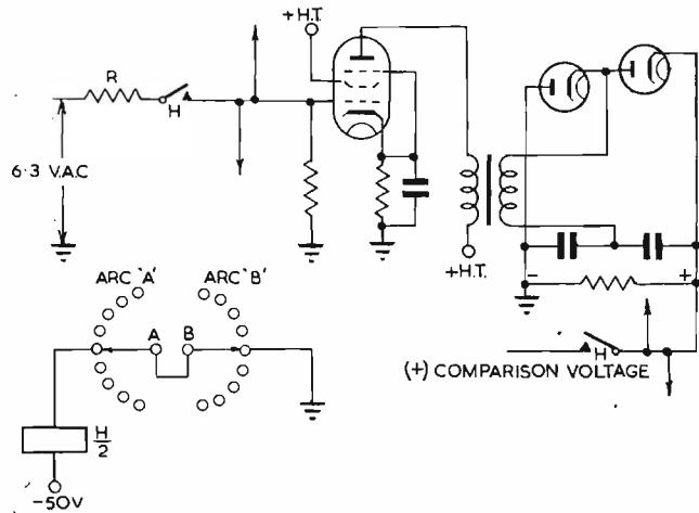
Fig. 7. Measurement of the heater voltage
