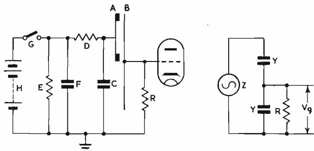
Fig. 2. Input and polarizing circuit
