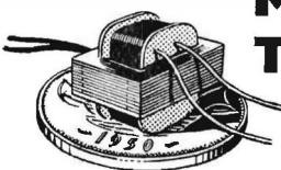
The high efficiency of these very small transformers is due to the special laminations, hydrogen annealed after stamping. Size of Transformer shown:  $\frac{3}{8}$ " x  $\frac{7}{16}$ " x  $\frac{1}{8}$ " dia. bobbin.
