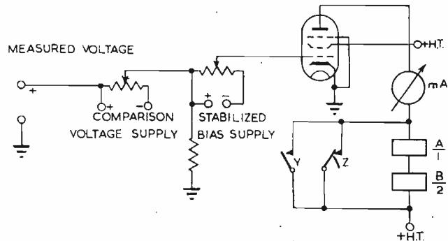
Fig. 1. Principle of the measuring circuit
