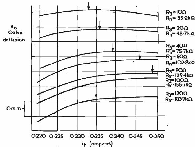
Fig. 4. Barth circuit—determination of minimum value of  $R_3$  necessary for balance (the vertical separation of the curves is arbitrary)
