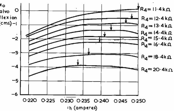
Fig. 6. Barth circuit—variation of balance point with  $R_4$
