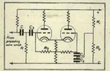
worst effects of leakage. At D.C. potentials, the resistance of the condenser C is much higher than that of the resistance  $R_{2}$  and the P.D. across the latter is so low that objectionable leakage cannot occur through the coupling condenser  $C_{2}$ and the grid leak  $R_{2}$ .
