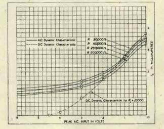
Fig. 6. (right). A.C. dynamic characteristics for R<sub>1</sub> 25,000 Ω.
