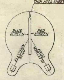
Fig, I, Diagram of double screen Cathode Ray Tube for viewing television images in two colours,
