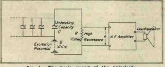
Fig. I. The basic circuit of the polarised electrostatic tone-generator.
