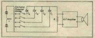
Fig. 2. Harmonic synthesis of complex musical tones by the addition of harmonically-related sine-waves of suitable amplitude
