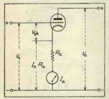
Fig. 1. Fundamental circuit. Vgk voltage between grid and cathode of amplifier. Ve input voltage to be measured. Va anode voltage. Ja anode current. Ra resistance of the anode circuit.
