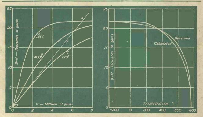
Fig. 2. Calculated Magnetisation curves of Iron according to theory of Paramagnetism. Fig. 3. Saturation Value of Iron in relation to temperature observed and calculated.
