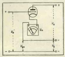
Fig. 3. Use of a boosting voltage (German Patent 690207) Vgo grid-cathode voltage for  $l_{\rm B}=0$  Vm voltage at an instrument connected as load of the anode circuit.
