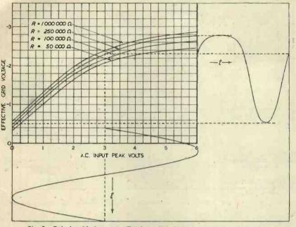
Fig. 7. Relationship between effective grid voltage Eg and A.C. input peak volts fer AC/HL for various values of grid leak.
