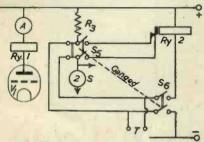
quired, one for relays with "make" contacts, and another for "break" contacts. It seemed to me that one universal instrument with a changeover switch incorporated would be more useful. Therefore, I append a modification of Mr. Bacon's circuit which appears as Fig. 4 in his article. My suggestion is that, instead of
