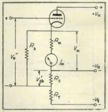
Fig. 4. Counterconnexion of Vgk. By the changes in cathod potential voltage changes at R<sub>B</sub> are caused through Rk corresponding to Vgk.
