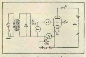
Fig. I (above). Apparatus for determining Ig-Eg characteristics.
