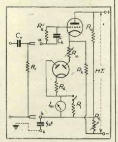
Fig. 6. Connexion for a.c. voltages rectified by a diode (German Patent 699719).
