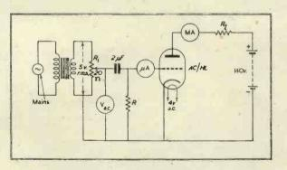
Fig. 5 (above). Determination of A.C. dynamic Eg-la characteristics.
