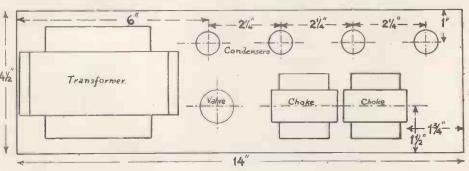
Fig. 6.-Layout of chassis-H.T. unit. The chassis is bent out of 16 g. aluminium with 2 flaps.
