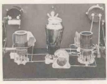
The doubler stage is quite straight-forward, but again, link couplings are fixed to the coil bolder and not the coil former. To reduce losses, mount the neutralising condenser in the wiring as shown.
