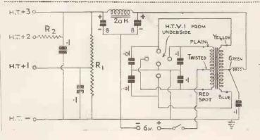
Fig. 1. — The fundamental circuit cannot be modified but resistances RI and R2 can be varied to give varying outputs.
