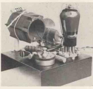
The split stator condenser shown is used as a single unit condenser, but it can be used as a split stator and then the anode coil must be centre tapped, but the anode by-pass condenser can be omitted.
