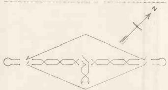
Fig. 2.—Diagram of horizontal rhombic antenna for receiving Alexandra Palace on 41.5 mc.
