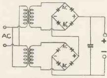
Fig. 8-Either vacuum valves or metal rectifiers can be used in a bridge circuit. In this instance metal rectifiers connected in series give a high output but require two HT transformers.
