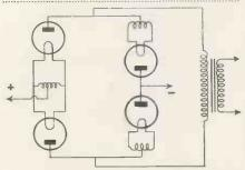
Fig. 4.—A bridge rectifier circuit using four halfwave valves enables twice the voltage output to be obtained.
