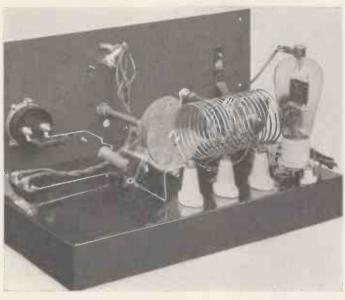
An air-spaced coil is used in the grid circuit of the T20. This is very efficient and also allows for easy adjustment of the link coupling which is merely plugged in to the centre of the coil.
