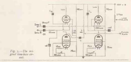
the circuit is running with the cathode earthed and the positive supply lead is, therefore, live to the chassis as in the conventional radio set.
