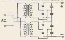
Fig. 6-Metal rectifiers are a distinct advantage in a voltage-doubling circuit owing to the fact that no delayed switching is required.
