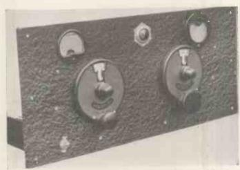
The sub-amplifier stage has the anode meter on the left-hand side and the grid meter on the right-hand side.
