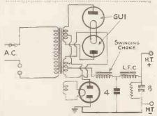
Fig. 3—Mercury vapour valves must only be used with a choke input circuit and need some means of delayed switching.
