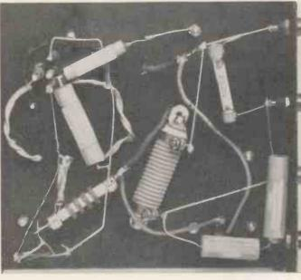
Here is the unit partially wired. It is quite simple to connect and the condensers and resistances need not be mounted. For those needing a greater number of tappings we sug-gest the use of a Bulgin group board to take the various resistances.
