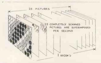
This diagram conveys the idea of how successive pictures can be thrown upon the screen and owing to the persistence of vision effect give an idea of continuity of motion.
