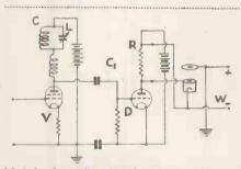
Method of coupling high-frequency amplifier to detector stage. Patent No. 465,405.
