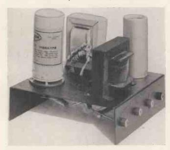
Although the unit is made up on a steel chassis there is no reason why it should not be made part and parcel of the battery receiver providing it is adequately screened. As shown, the vibrator is no larger than the average electrolytic con-denser and has a simple 5-pin base.
