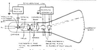
Fig. 2.—Schematic diagram of cathode-ray tube.
