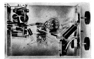
The Mullard AP4 valve is mounted in a special Bulgin low-loss holder.
