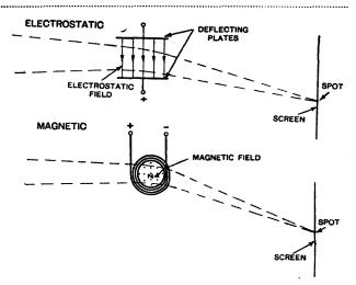
Fig. 4.—Diagrams showing the two methods of deflecting the cathode beam.
