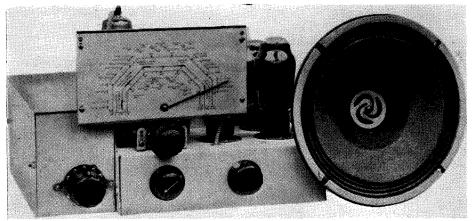
If the loud-speaker is mounted just above the tuning dial the receiver will have a very pleasing appearance. The wave-change switch has a positive action and is a part of the complete tuner.
