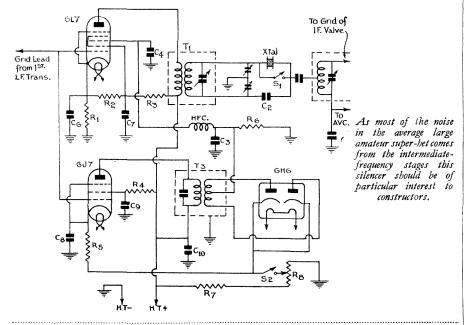
Silencing voltage is applied to the No. 3 injection grid, while the 6J7 and 6H6 are noise amplifier and rectifier respectively.
