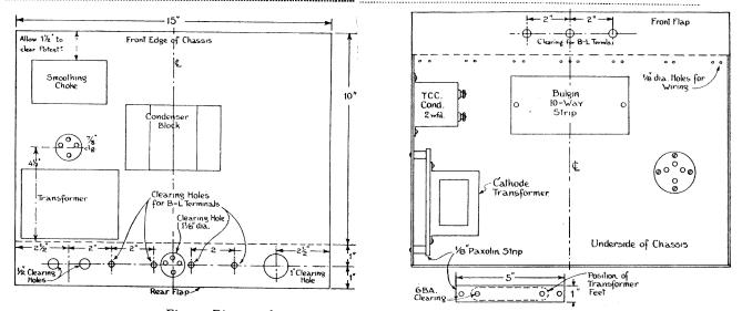
Fig. 3.—Diagrams of upper and under sides of base showing positions of components.
