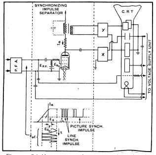
Fig. 11.—Suitable arrangements for separating the synchronising impulses from the picture signals in a receiver.
