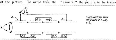
electrodes are connected in series with each other, so that their overall capacity is much reduced.
