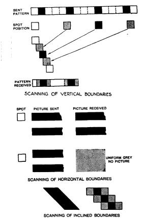
Figs. 8. and 9.—Diagrams showing the cause of aperture distortion.
