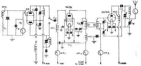
With only three stages this transmitter will handle an input of 1000-watts on 20-metres. It is also suitable for 10-metre operation with reduced power.
