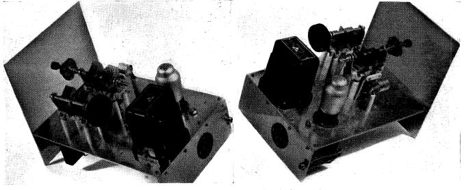
The large double-gang condenser in this illustration is for band setting.
