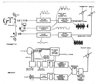
Fig. 6.—Schematic diagram of complete television system employing a disc transmitter and cathode-ray tube receiver.
