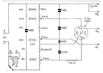
Fig. 1.—Circuit diagram of resistance chain.
