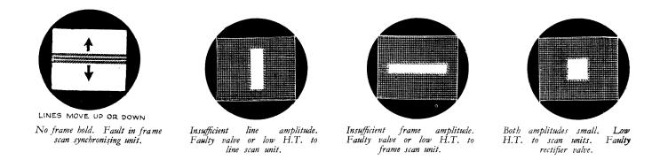
The sketches above are intended to give an approximate idea of the most obvious faults in a television receiver which are made apparent on the screen. They should not be interpreted too literally as in some instances the same effects might be produced in other ways.
