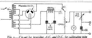
Fig. 2.— Cirvuit for providing A.C. and D.C. for calibrating tube deflections.
