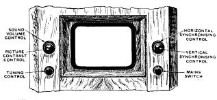
This drawing shows the normal controls on the G.E.C. receiver.
