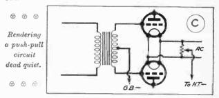
The "Hum-Dinger" total resistance, whilst not critical, should be selected for the best results. The usual standard value in A.C. valve circuits is a total resistance of 30 ohms, but other values from 6 to 200 ohms are available.
