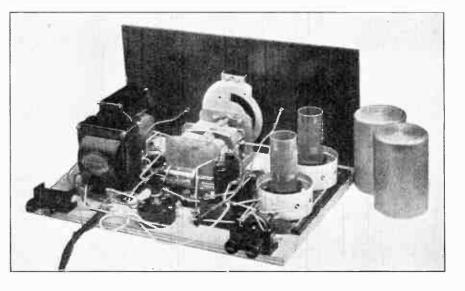
does normal service for this purpose. Depending upon what type of neon is used in the vision apparatus, so the voltage and current of the H.T. + connection will vary. My own tests were carried out with a Baird "Televisor." and the voltage of 200, giving a current of 25 milliamperes, suited admirably.
