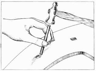
Fig. 2.-Correcting white lines on a disc by " closing " the hole with a light tup on a punch.
