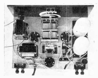
A good plan view of the completed receiver which can be compared with the wiring diagram of Fig. 3.
