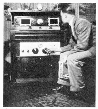
Another amatcur version of a dual vision and sound wireless receiver built into a cabinet complete with loud speaker and vision apparatus.
