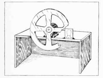
Fig. 1.-Testing discs by the use of a ground-glass screen secured by plasticine, the neon lump being replaced by an ordinary filament lamp.
