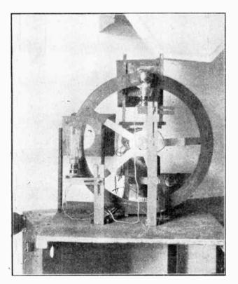
Looking at the back of Mr. Foster Cooper's vision apparatus. Both vertical and horizontal scanning may be employed, the separate neons for this purpose being clearly visible.
