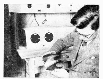
Examining the 60-line helical mirror drum employed in connection with Mr. Hewel's ultra-short-wave television experiments.
