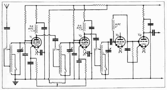
Fig. 1.—Mr. Barton Chapple's suggested scheme for the high-frequency and detector stages of the Tele-Radio Receiver. Volume control is secured through the medium of variable-mu valves, while a diode valve is to be employed to rectify the signals before they pass to the low-frequency amplifier.
