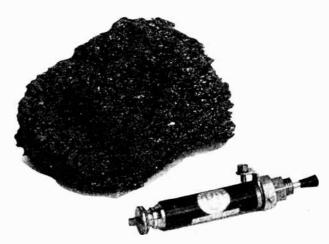
The designer of this receiver shows a preference for using a crystal detector in lieu of a valve. Above we see a large carborundum crystal and a standard permanent type.
