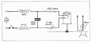
The scheme adopted for driving the motor—one which normally does duty in the home vacuum cleaner.
