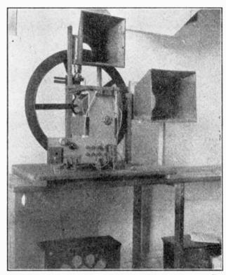
A front view of Mr. Foster Cooper's vision apparatus. By means of one switch he can bring either neon into circuit or alternatively pass the signals through a loud speaker for tuning purposes.
