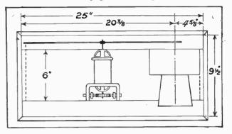
Fig. 4 .- .- . A plan of the baseboard lay-out supported on the plinth.
