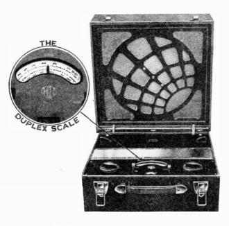
Showing the McMichael Duplex Four portable receiver. The pointer moves to the appropriate scale as the waveband switch is operated.
