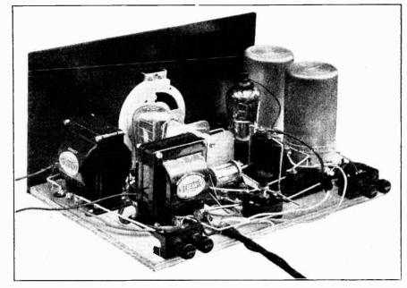
Looking at the back of the "Crystal" Three, showing the valves in place and the wiring completed ready for a reception test.
