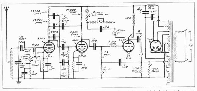
Messrs. E. J. and J. W. Holmes carried out a large number of experiments before deciding on their final vision wireless receiver circuit. The complete scheme is shown in the diagram above.
