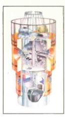
▲ Project Aries. This 16 ft. tall double-deck gondola is designed to attach to a massive Helium hot air balloon (I million cubic feet) which will travel at 80 m.p.h., 7 miles above the ground, in an attempt to complete a first non-stop round-the-world voyage. ATV
