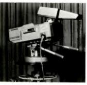
Pedestal-mounted colour cameras used in the studios and for normal outside-broadcast operations.
