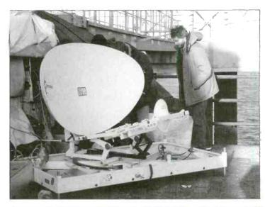
**Left:** ITN's mobile satellite ground station is used in remote areas to provide live transmission links.
