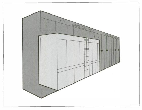
Left: Improvements in design have led to a significant reduction in the size of transmitters so that two modern transmitters can now be accommodated in the space previously occupied by one of two sets of the older equipments.
