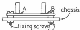
Fig. 4. Sketch showing how crystal holder is made from an old "Clix" valveholder.
