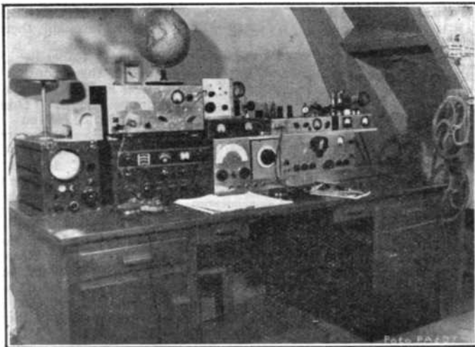
Inside the shack at PAoUN, famous VHF exponent. The hand-wheels at the right are used for rotating the beam aerials.
