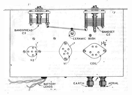
Fig. 2: Top of chassis layout.
