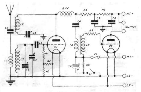
Fig. 1: Theoretical circuit.
