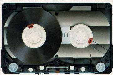
New exact pressure pad: thicker, with a strong spring, and twice as accurate as in conventional cassettes. It keeps the tape precisely perpendicular to the tape head. High precision cassette-shell: all dimensions are five times more accurate than specified by the I.E.C. Every component is built to micron-tolerances to minimise phase difference – time lag – between channels. The result: highly realistic stereo sound.
