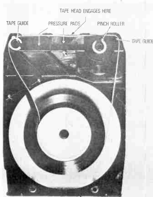
THE inside of an 8-track cartridge showing the continuous loop tape. Diagram courtesy of United Artists.
