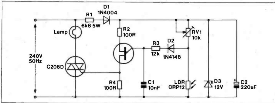
Figure 8. Circuit for an automatic lamp controller. The ORP12 photocell is used to control the UJT generator, triggering the triac on at dusk and allowing it to drop out at sunrise.
