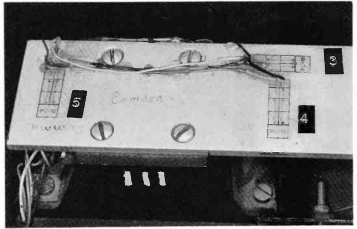
Photo 2. Strain gauges cemented to a beam. Numbers 3 and 4 are the 'active' gauges; number 5 is a dummy for compensating the bridge.
