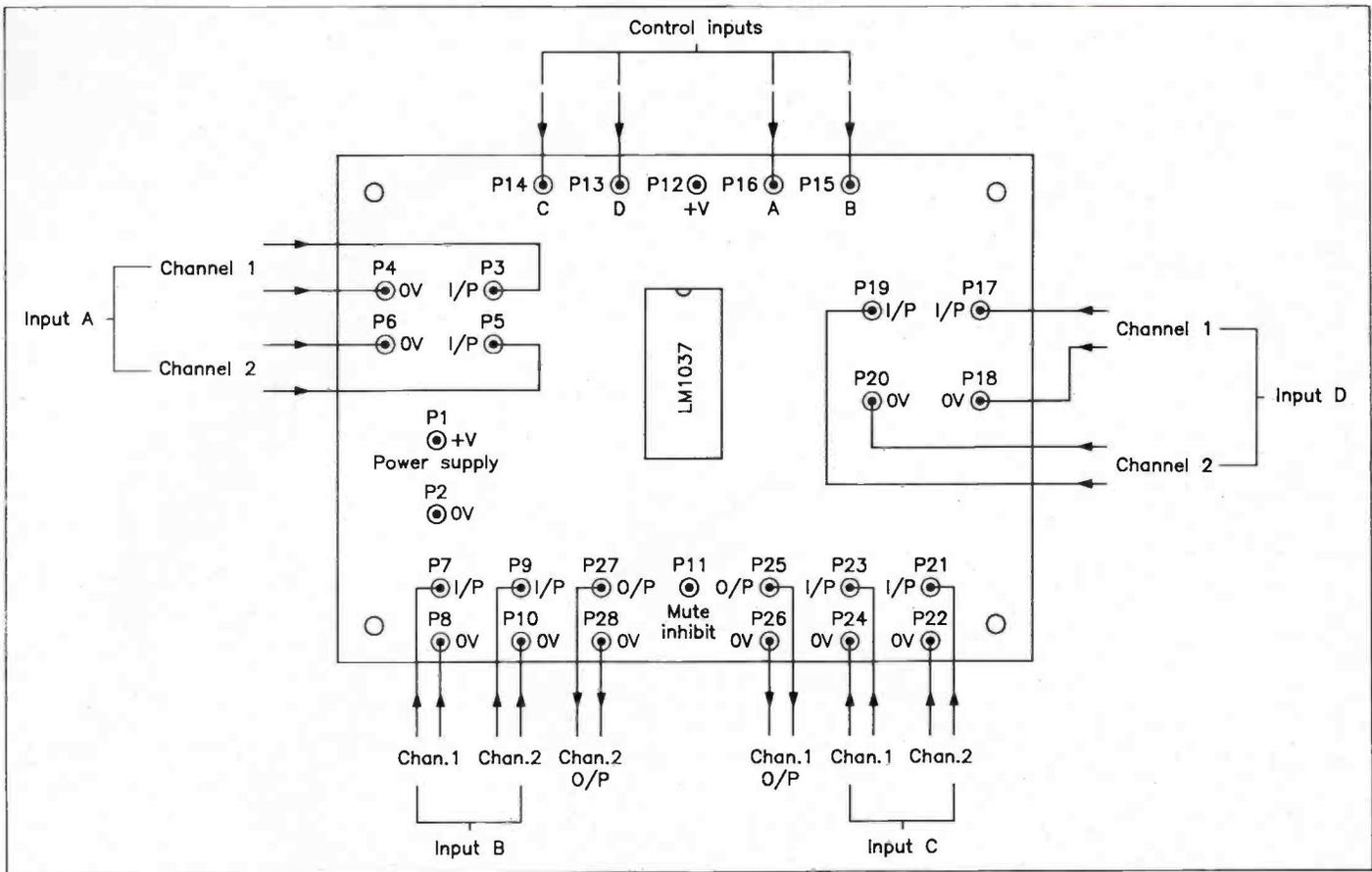
Figure 5. Wiring Diagram.
