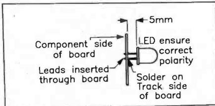
Figure 3. Mounting the LEDs.
