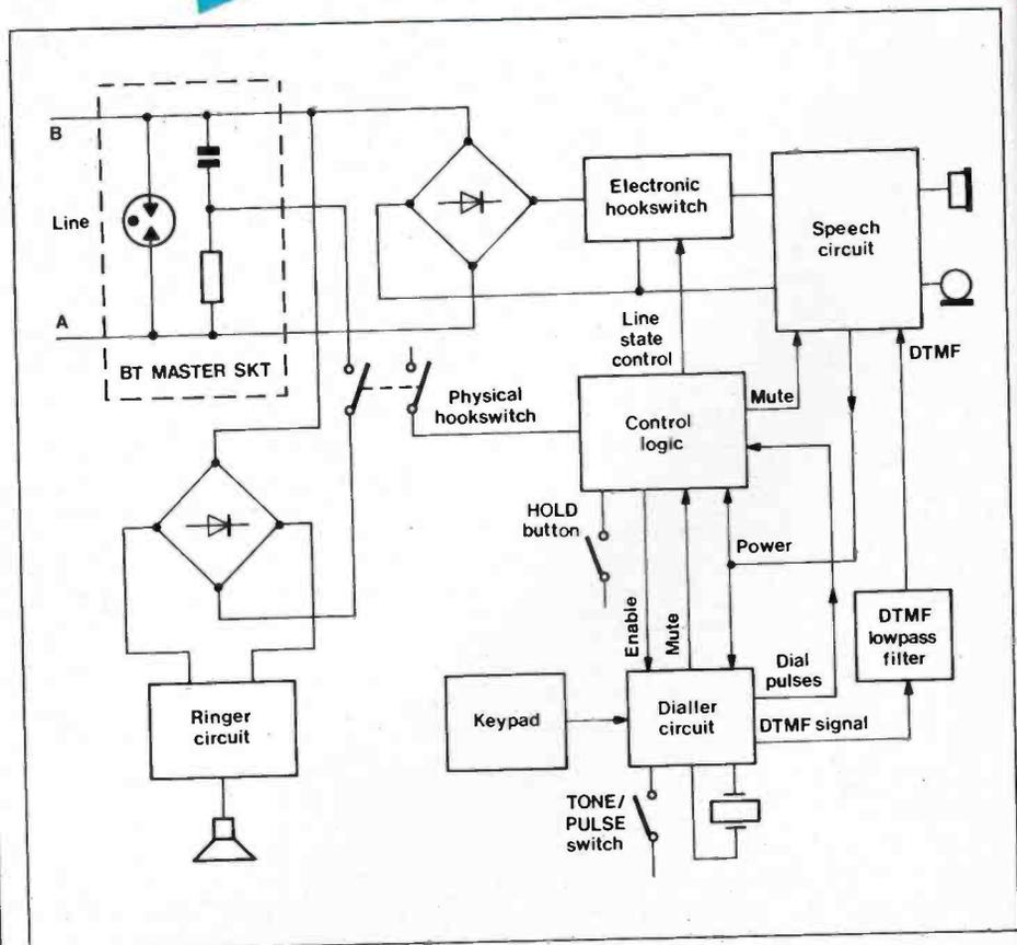
Figure 1. The elements of a modern telephone.
