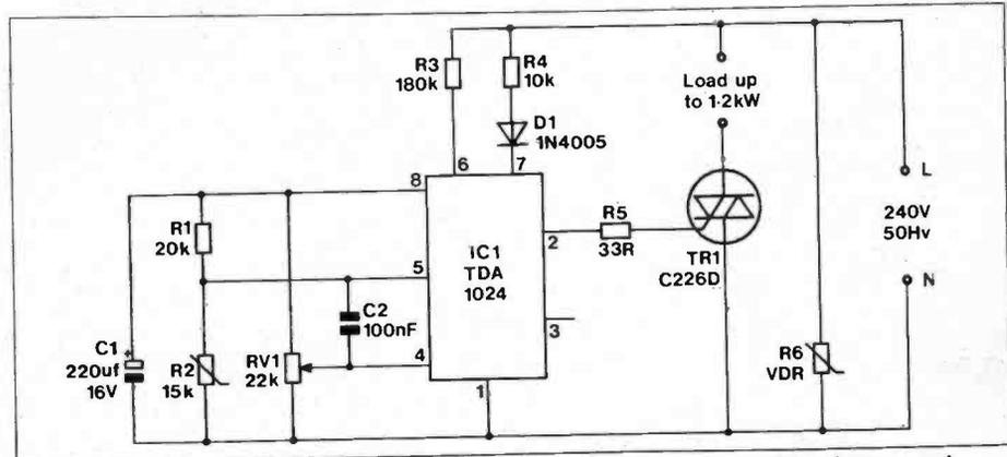
Figure 12. Practical circuit for integral cycle control using a readily available 'zero crossing detector IC'. A load up to 1.2kW can be controlled with this circuit. The C226D triac must be mounted on an adequate heat sink.
