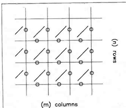
Figure 1. Part of an  $m \times n$  keyboard matrix, showing positions of keyswitches on the row/column intersections.
