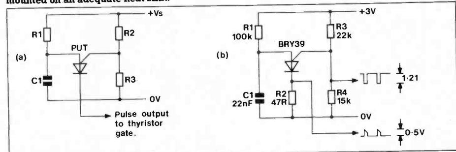
Figure 13. Using the PUT in the 'unijunction' mode, (a) general circuit for this mode, (b) a practical circuit for generating 1kHz pulses, needing a supply of only 3V. The value of 'u' is set by the values of R3 and R4 in the latter case [ $u = 15/(22 + 15) = 0.41$ ].
