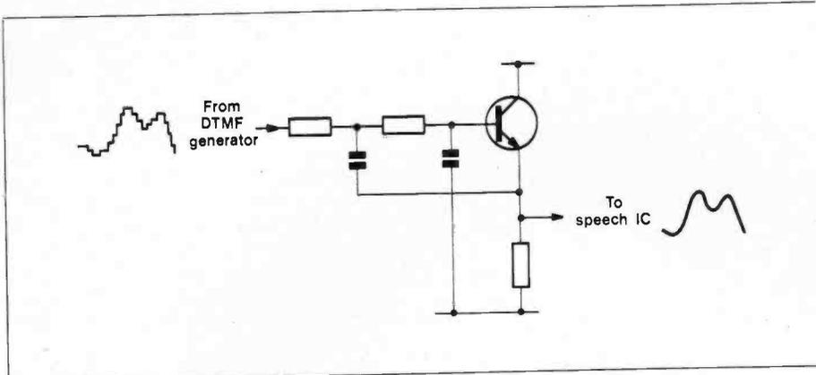
Figure 8. This simple lowpass filter is usually adequate to clean up DTMF signals.
