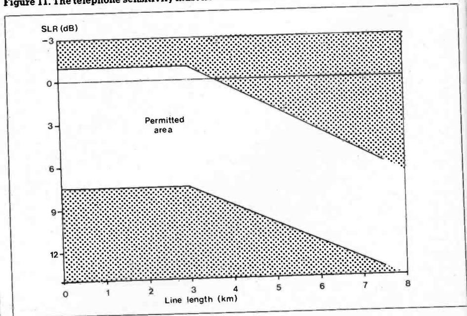
Figure 12. The send loudness rating (SLR) must be between specified limits.
