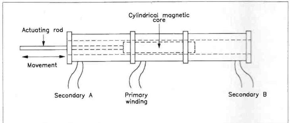
Figure 6. Basic construction of a Linear Variable Differential Transformer (L.V.D.T.)
