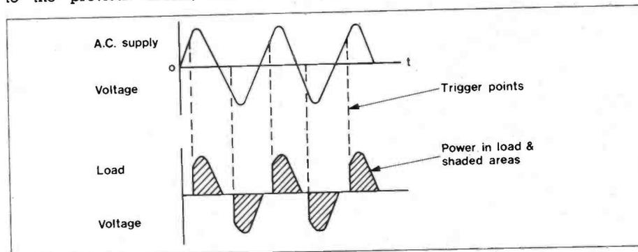
Figure 2. Power control using alternating current. Triggering is regular at the same point in each half-circle, giving a power to the load that is proportional to the shaded areas.
