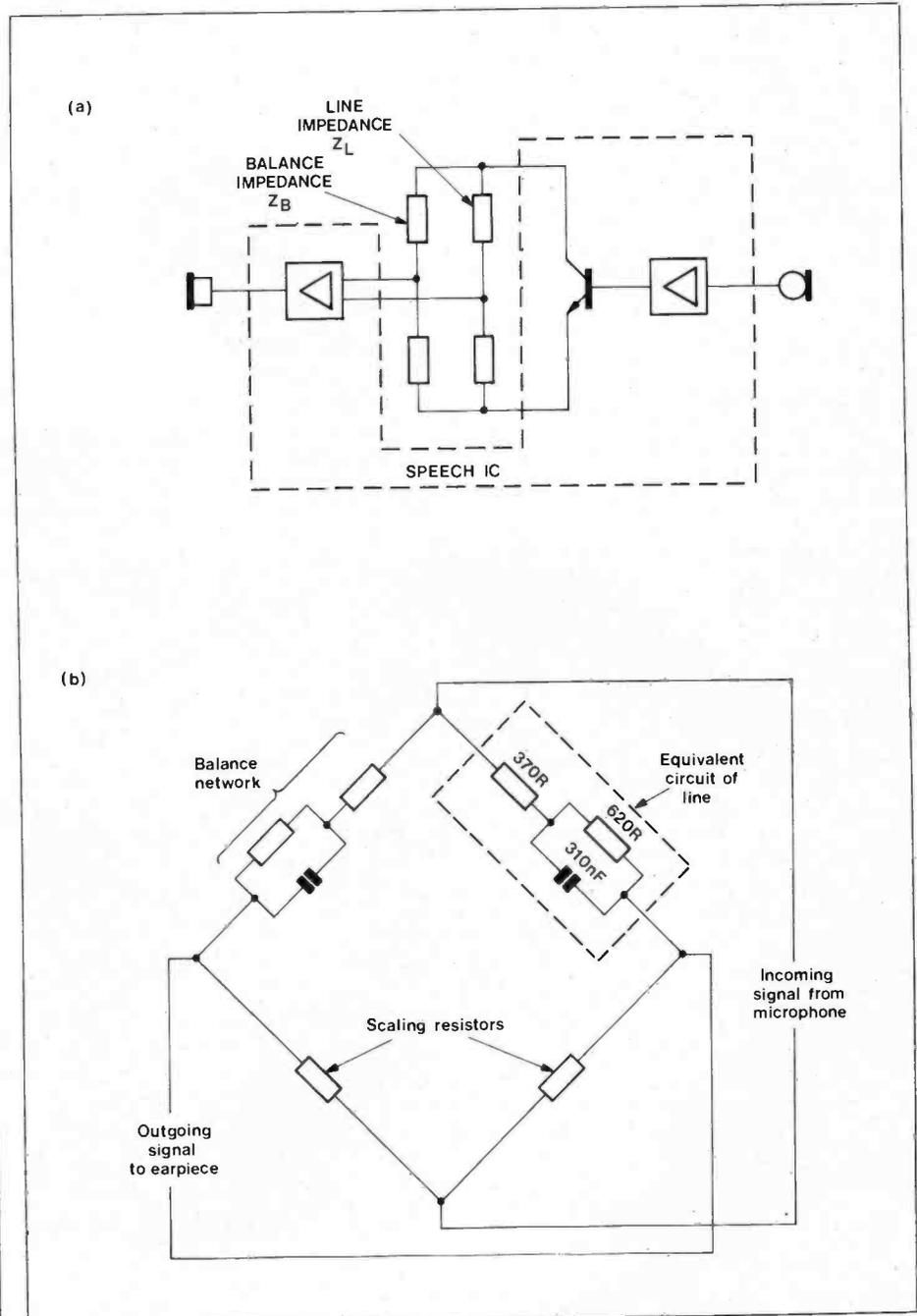
Figure 6. Sidetone balancing by means of a wheatstone bridge.
