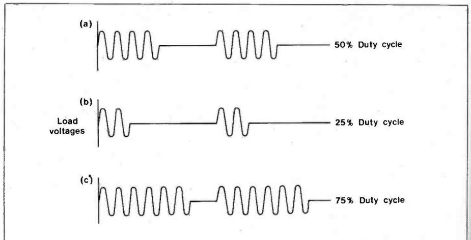
Figure 11. Waveforms to illustrate the principles of 'integral cycle control'. Power is controlled by the number of whole cycles supplied to the load, rather than by portions of cycles. As a result, load switching occurs when the supply voltage is zero.
