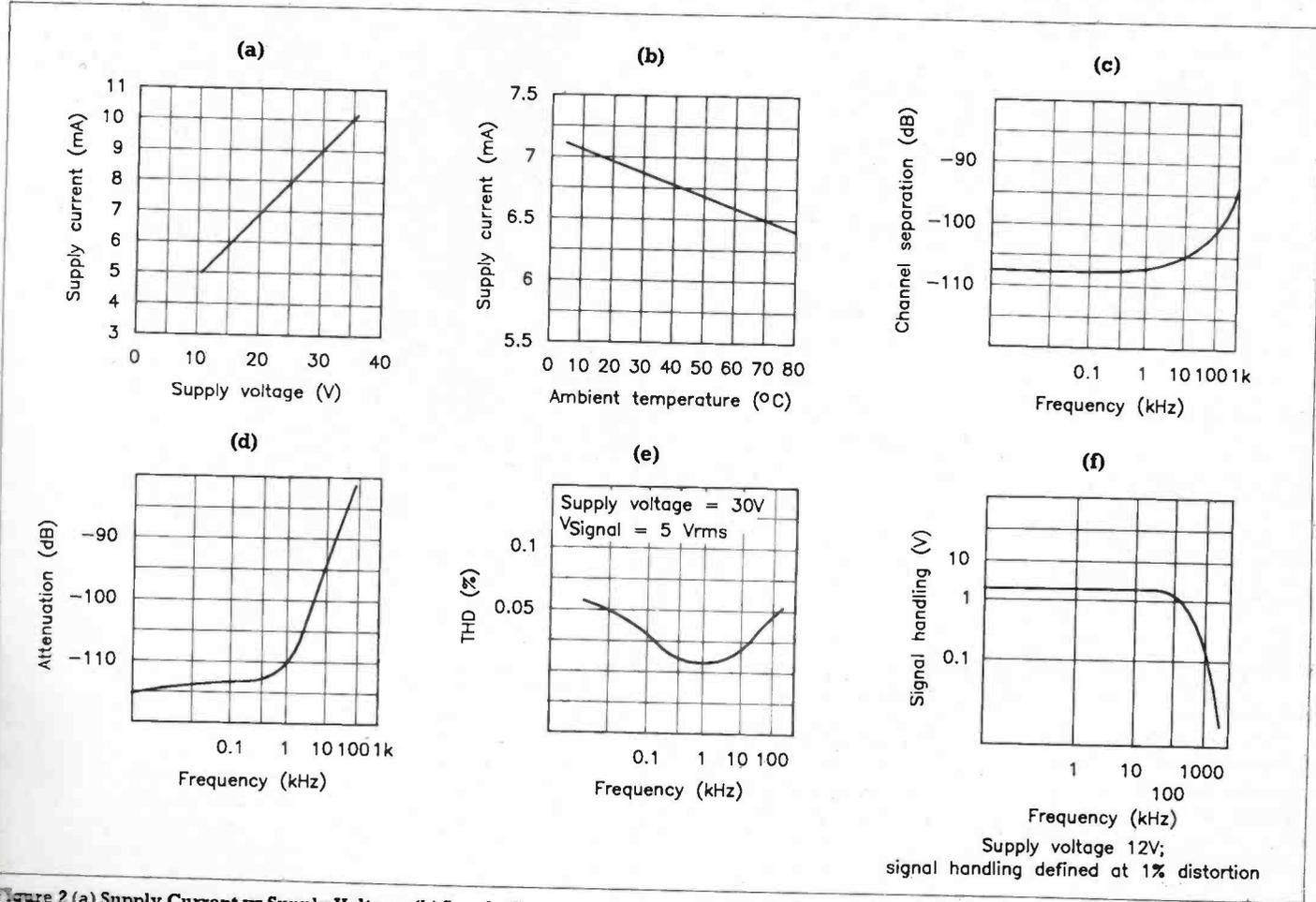
Figure 2 (a) Supply Current vs Supply Voltage, (b) Supply Current vs Temperature, (c) Channel Separation vs Frequency, (d) Attenuation of Selected Inputs vs Frequency, (e) THD vs Frequency, (f) Signal Handling vs Frequency.
