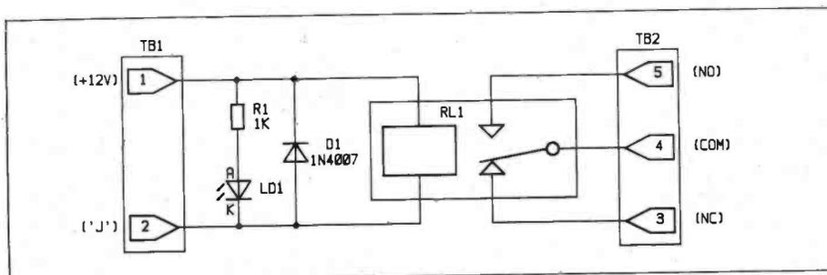
Figure 3. Circuit Diagram.
