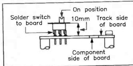
Figure 4. Mounting the Slide Switch.
