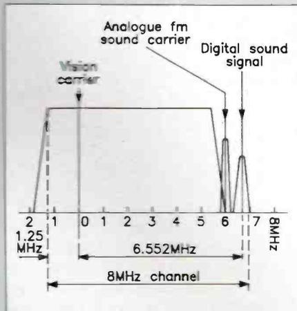
Figure 1. The frequency spectrum occupied by the NICAM 728 digital sound signal in relation to the vision and FM sound signals (UK System I). (Vertical axis not to scale.)
