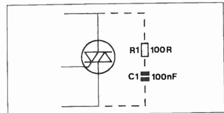
Figure 7. RC 'snubber' circuit to avoid accidental dv/dt triggering when the load is inductive.
