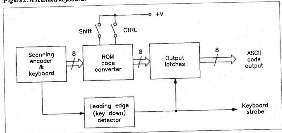
Figure 3. A scanned keyboard with ROM to store the ASCII codes.
