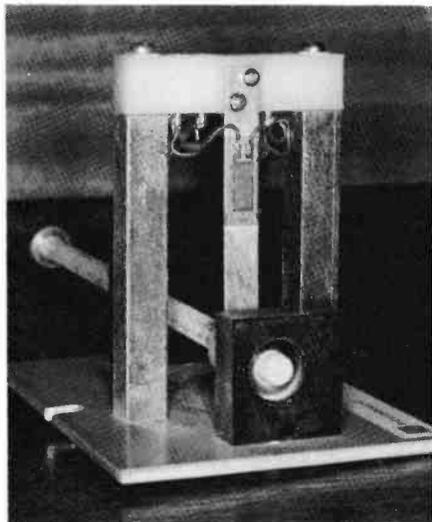
Photo 1. A single strain gauge attached to a member under test in loading jig.
