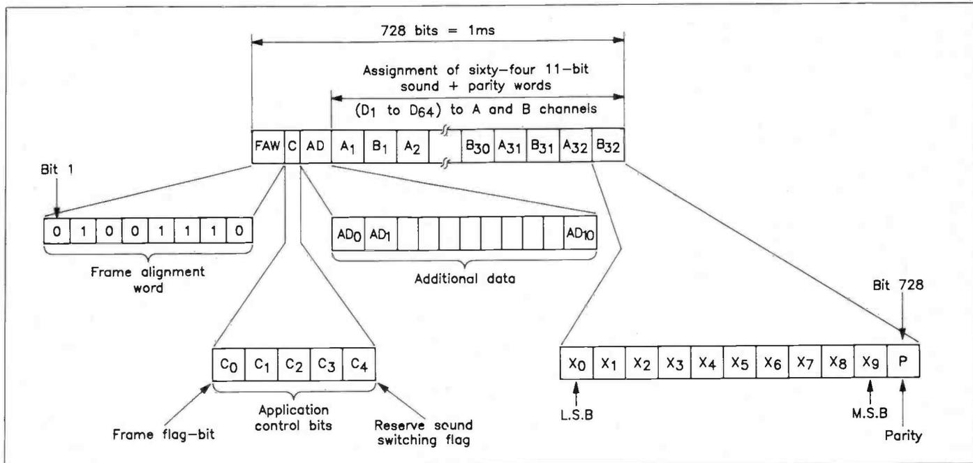
Figure 6. Structure of 728 bit frame containing stereo sound (before interleaving).
