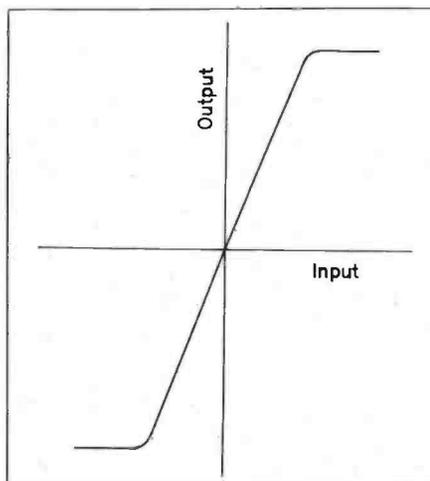
Figure 1c. Transfer characteristic showing peak clipping.
