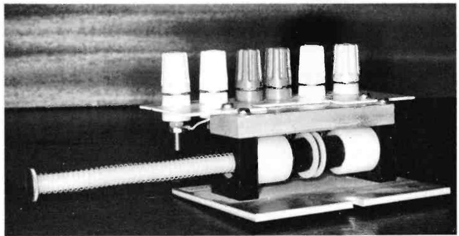
Photo 3. Example of a linear variable differential transformer (L.V.D.T.). The 'displacement' input is via the spring-loaded shaft.
