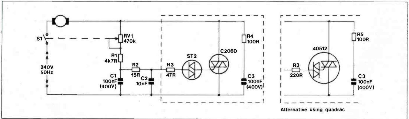
Figure 10. Two possible circuits for controlling the speed of a small universal motor. Either a diac/triac combination or a quadrac can be used.
