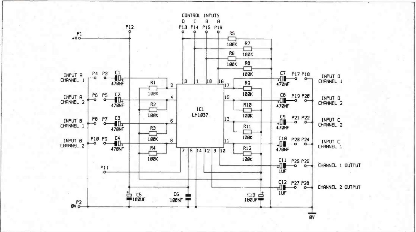
Figure 3. Circuit Diagram.
