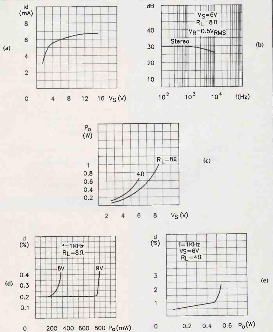
Figure 2. Electrical characteristics. (a) Quiescent current vs Supply voltage. (b) Supply voltage rejection vs Frequency. (c) Output power vs Supply voltage (THD = 10%,  $f = 1kHz$  stereo). (d) Distortion vs Output power (stereo). (e) Distortion vs Output power (stereo).
