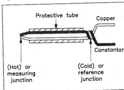
Figure 4. Essential construction of a copper/constantan thermocouple.
