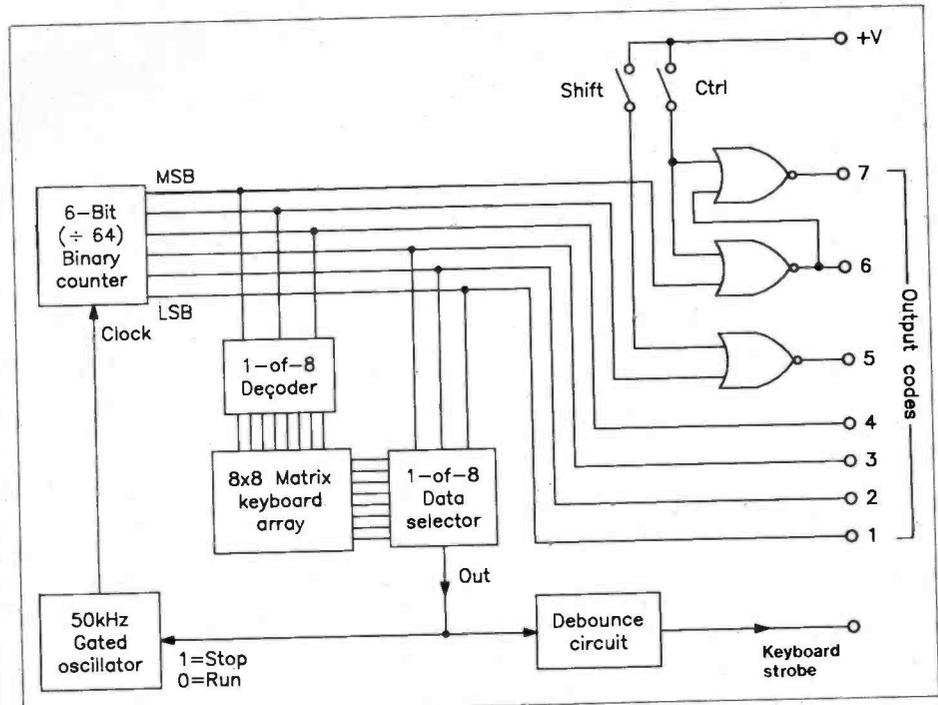
Figure 2. A scanned keyboard.
