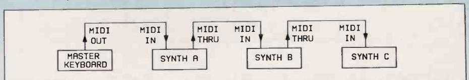
Figure 1. Connecting synthesisers using MIDI chain.
