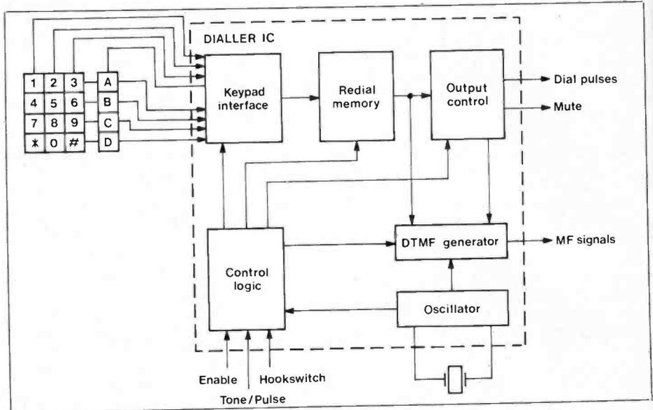
Figure 7. A typical dialler circuit.
