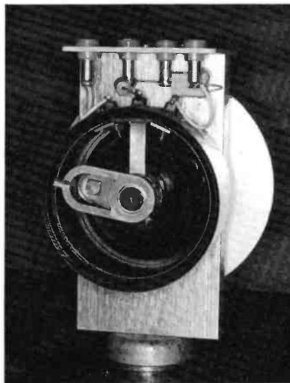
Photo 4. Example of large wirewound (rotary) potentiometric transducer.
