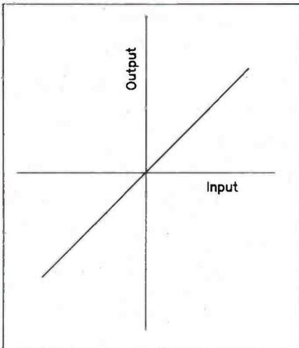
Figure 1a. Linear transfer characteristic.
