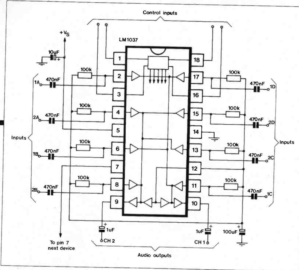
pins (pin 7) of the devices together and connecting the two pairs of output pins (pin 9 and pin 10) in parallel. It should be noted that only one output capacitor is required for each channel.
