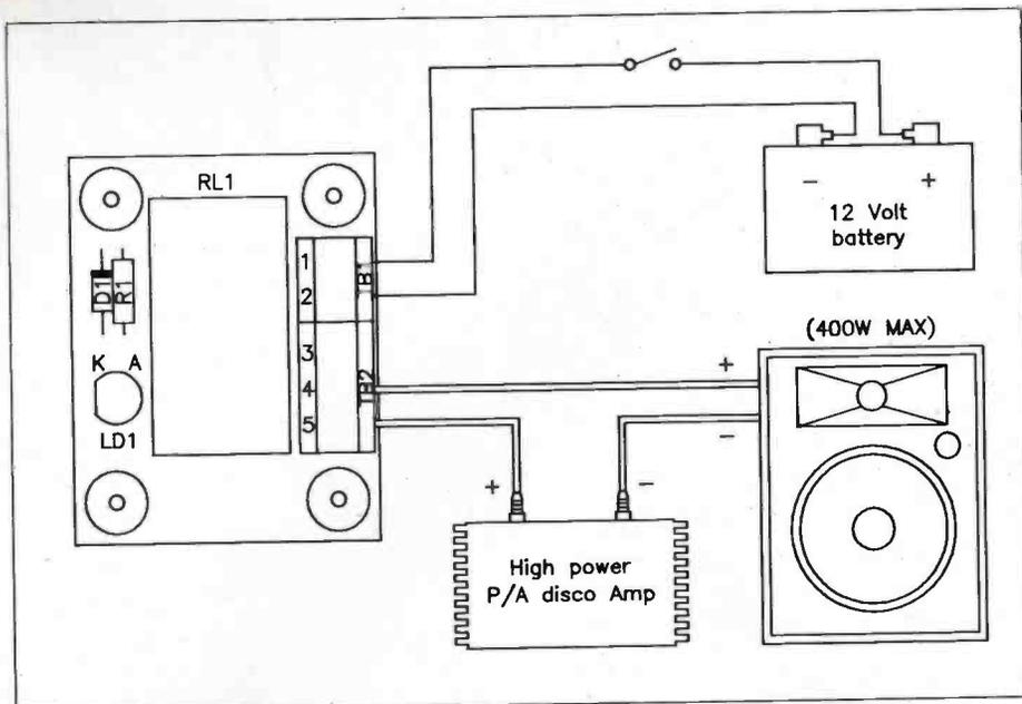
Figure 2. Wiring for high power speakers.
