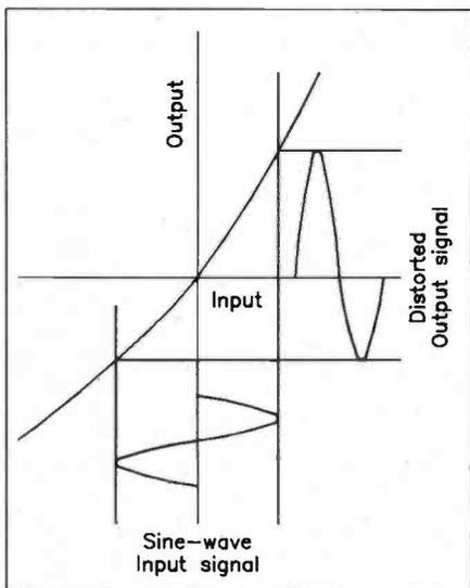
Figure 1b. Curved transfer characteristic showing distorted output from sine wave input.
