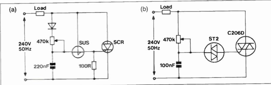
Figure 5. (a) Half-wave phase-control circuit using SUS to trigger a SCR, (b) full-wave phase-control circuit using diac to trigger a triac. Both circuits use single time constants.
