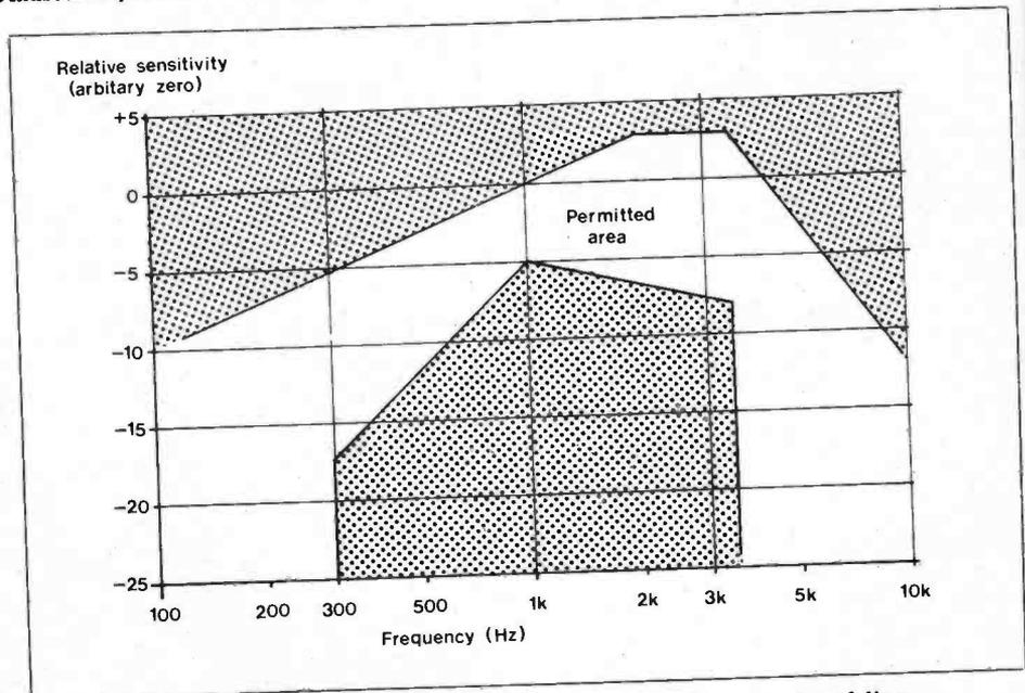
Figure 11. The telephone sensitivity must lie within these limits for a zero-length line.
