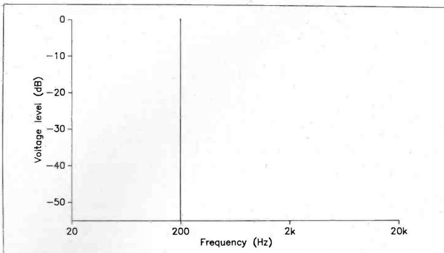
Figure 2a. Spectrum of a 200Hz sine wave signal.
