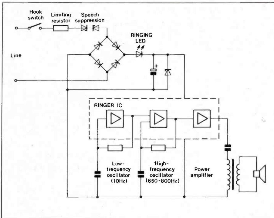
Figure 2. A typical ring detection circuit.
