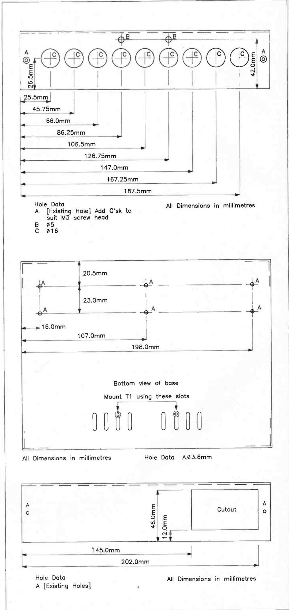
Figure 7. Box drilling details.
