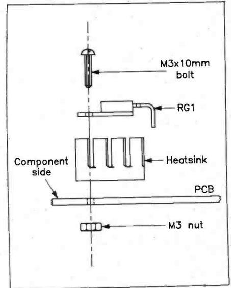
Figure 6. Assembly of regulator and heatsink.
