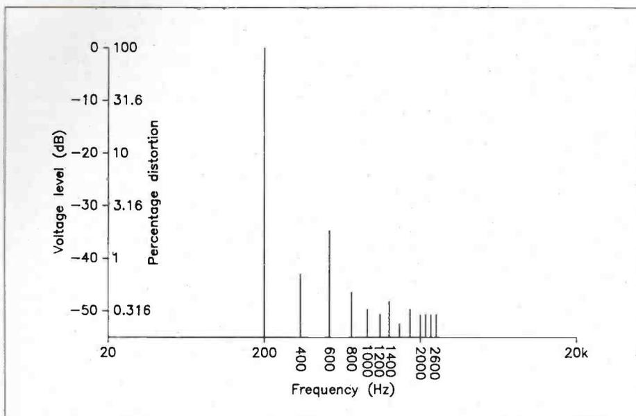
Figure 2b. Spectrum of amplifier output with 200Hz sine wave input showing harmonics up to the 13th.
