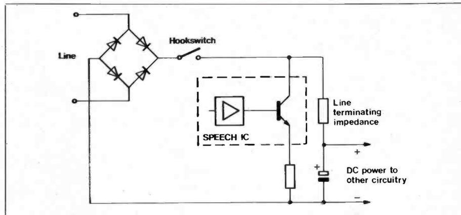
Figure 4. Line impedance matching and power extraction.
