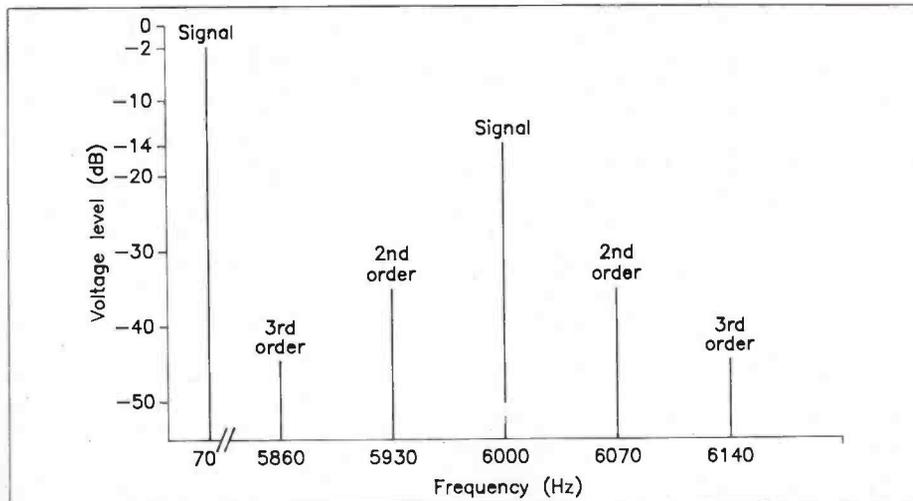
Figure 2f. Spectrum of two-tone (inter)modulation products (input 70Hz and 6kHz with amplitude ratio 4:1).
