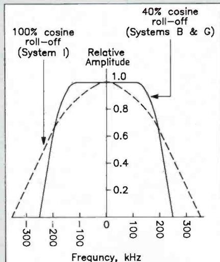
Figure 2. Spectrum shaping (due to combined transmit/receive data-shaping) for System I and Systems B and G.
