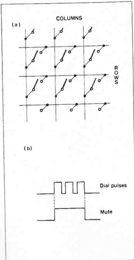
Figure 9. (a) Keypad switches arranged in a matrix. (b) The mute output provides a blanking pulse during dialling.
