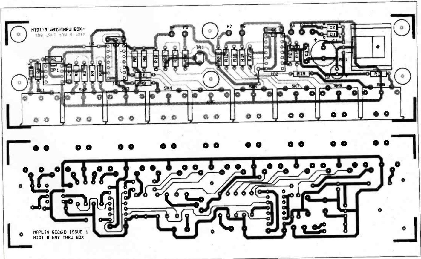
Figure 5. PCB legend and foil pattern.
