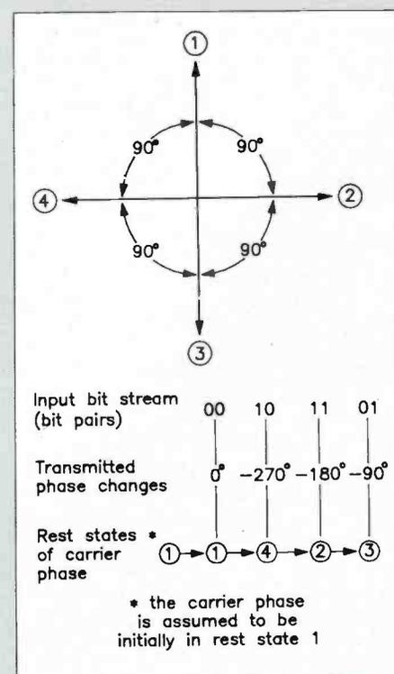
Figure 3. The four rest-states of carrier phase of the digitally modulated carrier for NICAM 728 are 90° apart.
