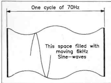
Figure 2e. Waveform of output from two-tone (inter)modulation test signal (70Hz and 6kHz) with 70Hz and harmonics filtered off. Result is an amplitude-modulated 6kHz sine wave, x-deflection for the display is the 70Hz input signal.
