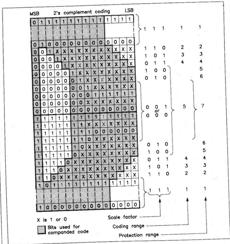
Figure 5. Coding of companded sound signals.
