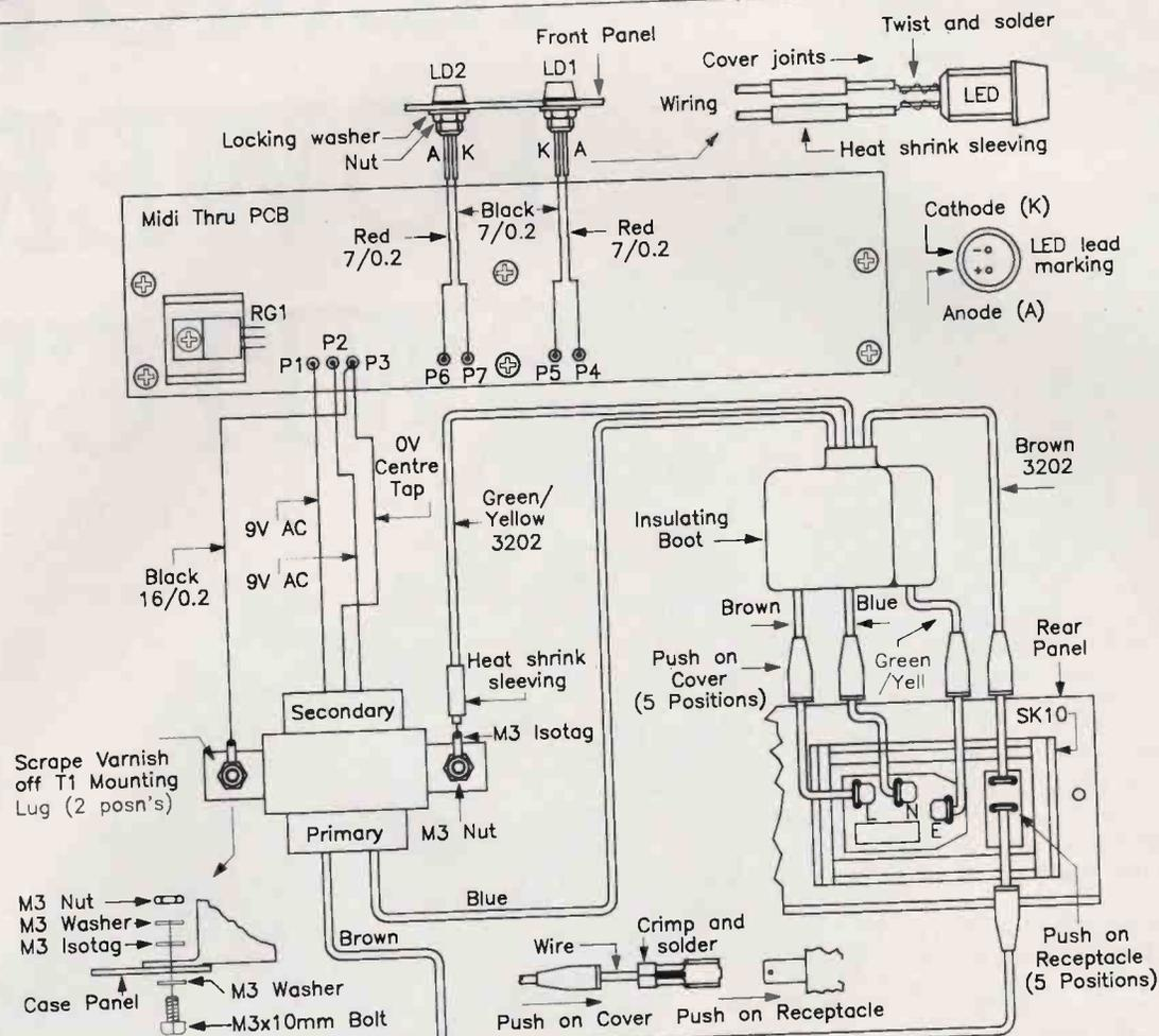
Figure 8. Wiring and assembly diagram.
