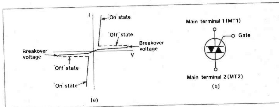
Figure 1. The triac, (a) characteristics, showing bi-directional nature and (b) circuit symbol.
