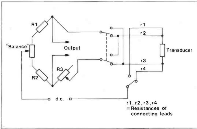
Figure 5. The Mueller bridge, used when long connecting leads are involved.
