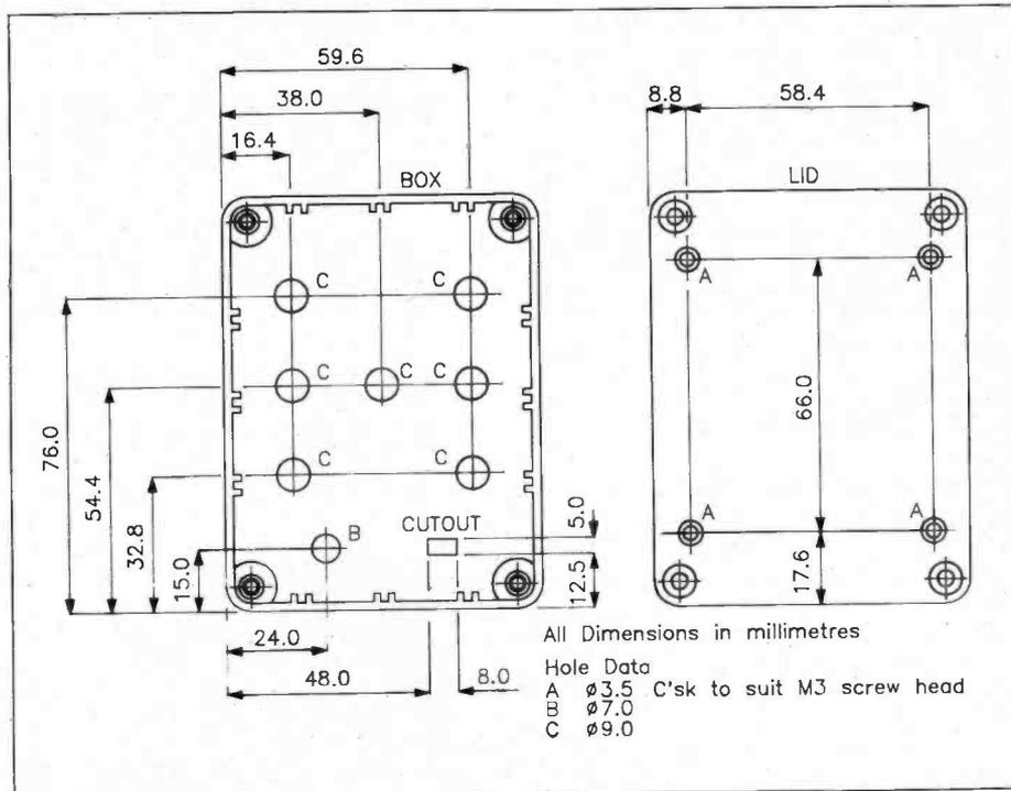
Figure 5. Drilling Details.
