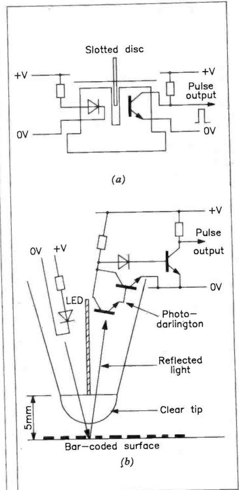
Figure 11. (a) Principle of optical coupling applied to the generation of pulses by a rotating, slotted disc (e.g. to measure engine speed), (b) Using an LED and a photo-Darlington amplifier to read bar codes.
