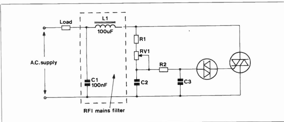
Figure 6. Double time-constant phase control circuit, with filter (L1 and C1) to eliminate RFI.
