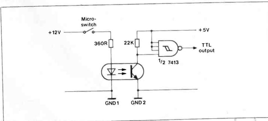
Figure 9. Using an opto-isolator to interface a microswitch to a digital circuit, avoiding 'ground noise' problems.
