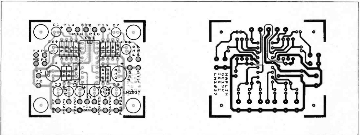
Figure 4. PCB Layout.
