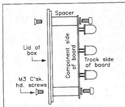
Figure 6. Installing the PCB.
