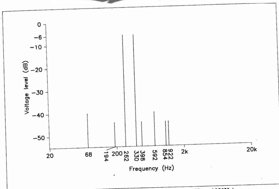
Figure 2c. Spectrum of two-tone intermodulation products (input 262Hz and 330Hz).
