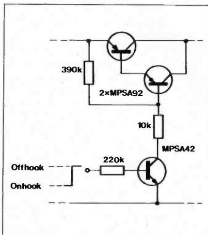
Figure 3. The hookswitch is often realised like this.
