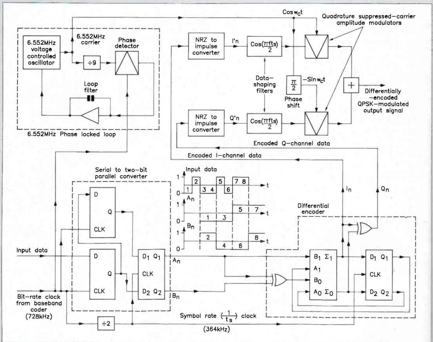
Figure 4. NICAM 728: Block diagram showing the processes of differential encoding, data-signal shaping and modulation at the transmitter.
