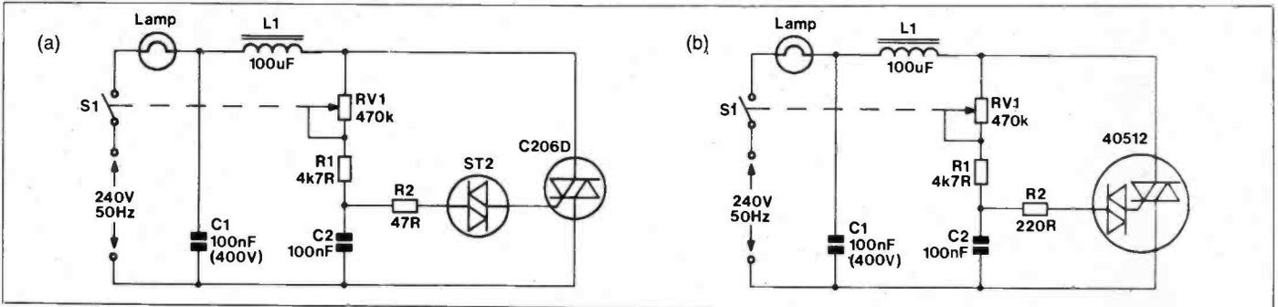
Figure 9. Two alternative lamp dimmer circuits, (a) using a diac and triac, (b) using a quadrac.
