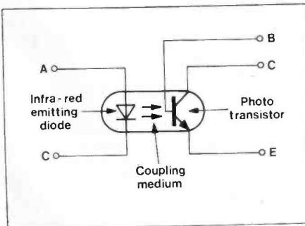
Figure 8. The optically-coupled isolator (opto-coupler or opto-isolator).
