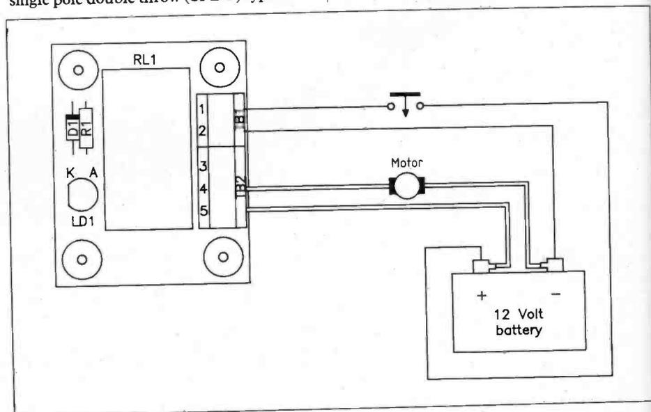
Figure 1. Wiring diagram for motor/most applications.
