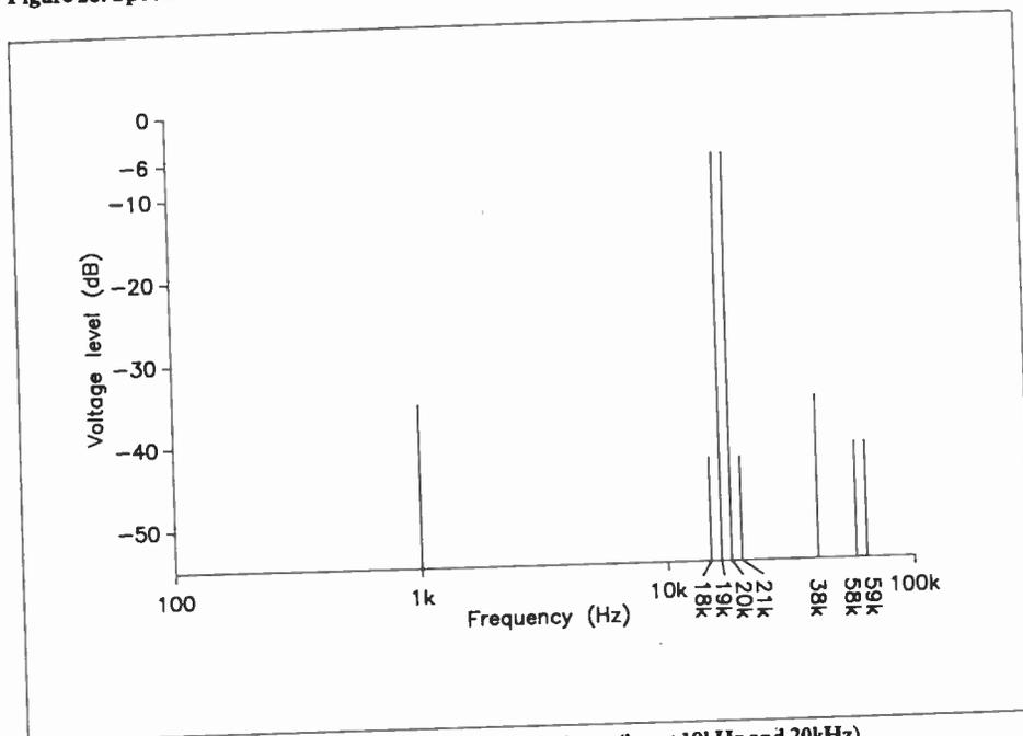
Figure 2d. Spectrum of two-tone intermodulation products (input 19kHz and 20kHz).
