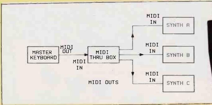
Figure 2. Connecting synthesisers using MIDI Thru' Box.
