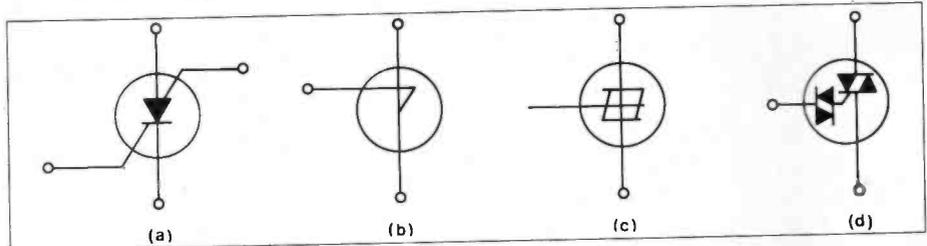
Figure 4. Circuit symbols for four members of the thyristor family. (a) SCS (b) SUS (c) SBS and (d) quadrac.
