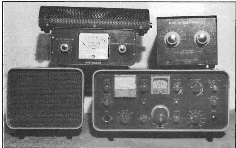
The KW2000A, with matching speaker/PSU, SWR bridge, 'E-ZEE' match and dummy load
