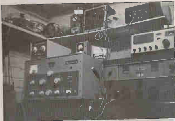
G3XTT in 1972. Heathkit DX-1000 transmitter, AR77 receiver, and Heathkit 2m transceiver (plus assorted junk!)
