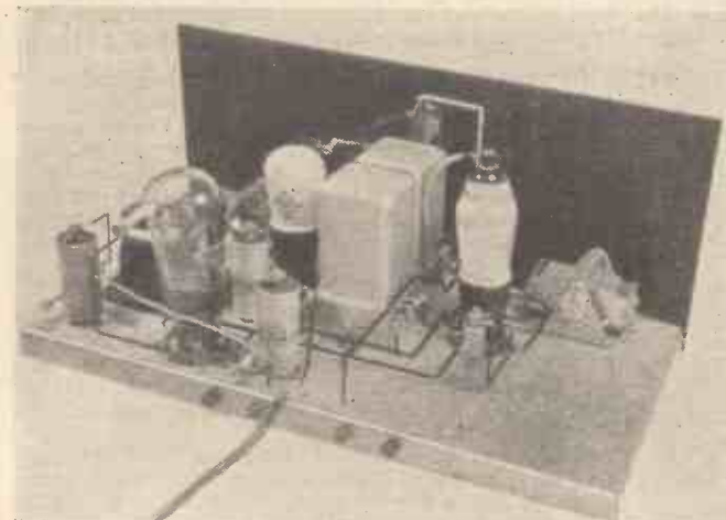
Another view of the set with the three valves in position ready for preliminary testing before inserting in cabinet
