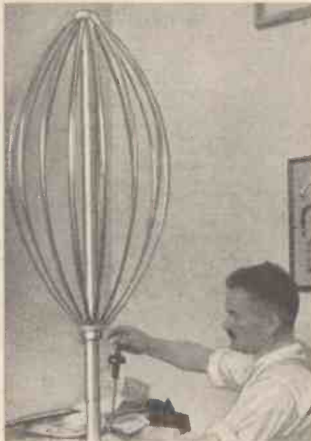
Gullstrand photo Novel type of receiving aerial shown at the Berlin Radio Exhibition. It is used in conjunction with a screened download
