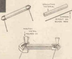
How Dubilier resistances are made. The mould shown in the lowest sketch is simply the artist's impression of what the inside The cone piece corresponding to the funnel is knocked off shape is like.
