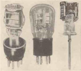
(Left).—Internal construction of the Marconi QP21 cutput valve. (Centre and right).—Two views of the 362 class-B battery valve
