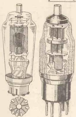
Mullard type DB26 26-volt output (Right): Ostar-Ganz B2 A.C./D.C. (Left): valve. valve for universal mains sets
