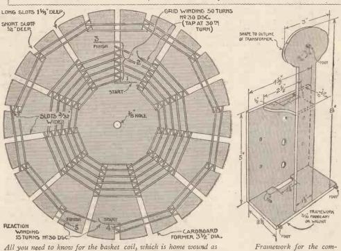
All you need to know for the basket coil, which is home wound as explained in the article. Note the double series of slots: one for the tuning and the other for reaction. This sketch is actual ize
