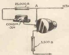
Fig. 2.—Addition of a .004-microfarad by-pass condenser to give mutual balance
