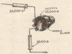
Fig. I .- Use of three resistances in series, two fixed and one variable
