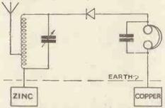
Using two separate earths to bias a carborundum crystal detector
