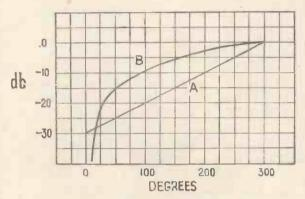
Fig. 3.—A shows decibel or logarithmic volume control and B shows ordinary uniform volume control
