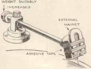
How an extra horseshoe magnet can be fixed to an old pick-up to increase its sensitivity
