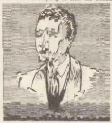
Faulty angular positioning of the holes results in the picture being stepped and radial faults are revealed by black or white lines according to whether the holes are too far apart or too close together
