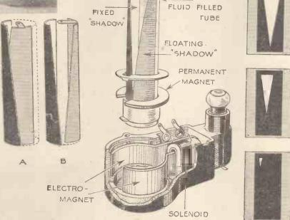
How the Weston tuning indicator is arranged. At A the fixed and moving "shadow pieces" are in the maximum position and at B they are in the minimum position.
