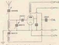
Circuit of simple short-wave super-het converter
