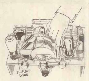
"In some cases the aerial wire itself is housed in the middle of an earthed tube made up of braided wire"
