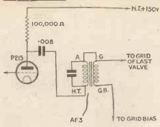
Fig. 2.—Coupling between second and third low-frequency valves
