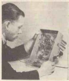
Note the workmanlike appearance of the chassis-built Universal High-voltage Radio converter for A.C. or D.C. mains
