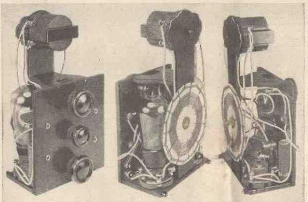
How the components are arranged on the wooden framework is very clearly shown by these three photographs. low-frequency transformer is screwed to the shaped end-piece. Note the position of the basket coil
