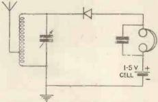
Inserting an old grid cell in the return headphone lead for crystal bias
