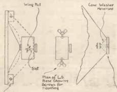
Side Elevation Enlarged View of Armature (Dotted Line Shows Plywood Chassis) Showing Method of Mounting
