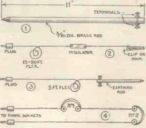
Fig. 1.—Earthing rod to go inside attaché case. Fig. 2.
