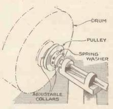
Fig. 3.—A type of mechanical filter favoured in Germany; it employs a slipping clutch
