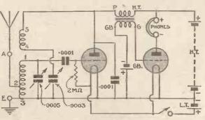
Theoretical circuit of the Hiker's Portable, showing the detector with reaction and the transformer-coupled low-frequency stage
