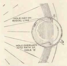
This diagram shows in an exaggerated manner the faults which may be present in a disc
