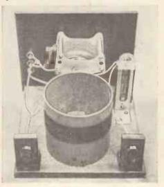
There is an extension control on the verticallymounted preset condenser
