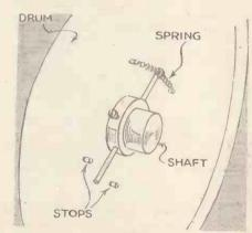
Fig. 2.—The movement of the drum or visor is controlled by two tension springs attached to an arm on the centre boss
