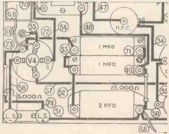
How the wiring is altered for pentode output. A complete full-size blueprint can be obtained for 1s. 6d., post paid; No. AW433 with triode output and No. AW433a with pentode output
