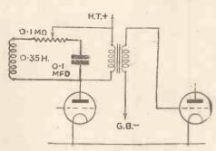
Fig. 1.—Tone control applied to circuit with direct transformer connections
