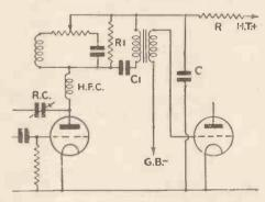
Fig. 3.—Tone-control as applied to a parallelfeed circuit
