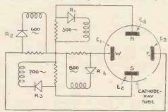
Fig. 3.—Cathode-ray receiver
