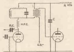
Fig. 2.—Circuit with capacity reaction
