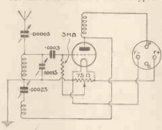
Circuit of simple short-wave plug-in adaptor
