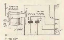
Theoretical circuit of the whistle filter—which can also be used as a wavetrap
