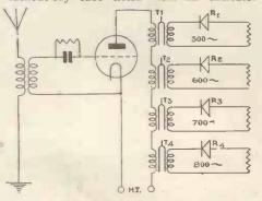
Fig. 2.-Receiver circuits arranged with tuning-fork selectors
