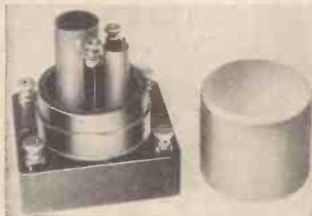
Top view of the Graham Farish unit, showing the compact arrangement of the two condensers and two resistances.
