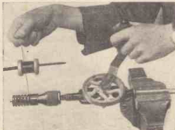
Winding the fine wire into the six slots of the ebonite former is quite simple if you adopt this system. Turn the choke former in a twist drill held in a vice and slowly unwind the reel of wire over a pencil or screwdriver
