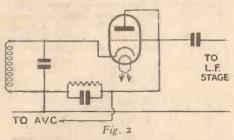
The only difference between this and the ordinary diode circuit is that here it is the grid grid of the tuning coil that is earthed and not the cathode end, as may easily be seen by re-drawing the circuit as in Fig. 3.
