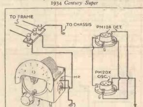
Connections for a two-terminal frame aerial on the
