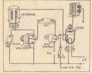
How to fit the 1934 Century Super with a radiogram switch to change over from radio to pick-up at will. Nearly everybody will want to make this improvement!
