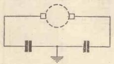
Fig. 2—A couple of fixed condensers shunted across the motor brushes, as shown above, will prevent trouble due to sparking
