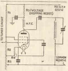
Fig. 4.—Recommended circuit for obtaining screen-grid bias voltage for VP4 screened pentode
