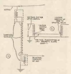
Fig. 2-(a). Arrangement of shielded lead-in and (b) the principle of impedance matching
