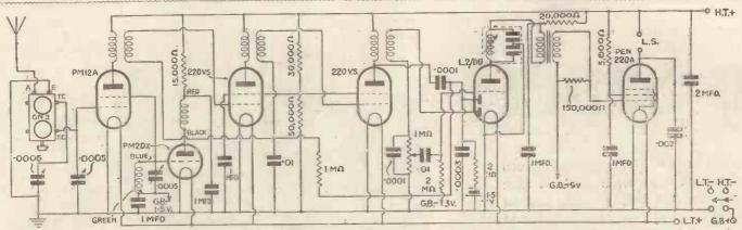
Circuit of the 1934 Century Super, of which the valve combination is first detector, oscillator, two intermediate stages, second detector and pentode
