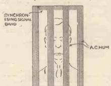
Fig. 1—This sketch gives an idea of the appearance of the picture when interference from A.C. mains is being experienced
