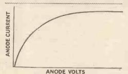
Fig. 2.—General form of characteristic curve of high-frequency pentode
