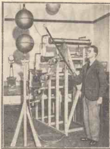
To test lightning arrestors and lines the Post Office employs artificial lightning apparatus. It can generate 250,000 volts!
