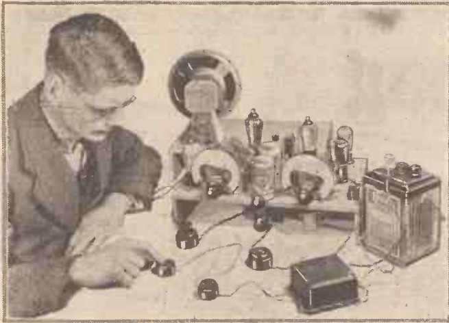
Trying out the Etherdyne with Bulgin plugs and wall jacks, wired on the twin-wire extension system
