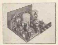
Circuit: S.G., D., R.C., Trans. (Battery). Price of set, less valves, £3 5s.; complete with valves and cabinet, £5 4s. 3d.
