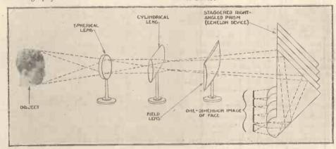
Fig. 1. This pictorial diagram gives some idea of how the two-dimensional picture area is turned into a line of light through a staggered series of prisms, arranged in echelon formation
