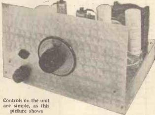
the detector oscillator. Well, firstly, you do get a decided increase in amplification, even down to 17 metres; secondly, the extra valve levels the load on the detector-oscillator, so that blind spots are wiped out; and, thirdly, it eliminates most of the bugbear of second-channel interference—that is to say, it reduces "images" of the fundamental signal frequency that tend to appear round the dial with simpler circuits.
