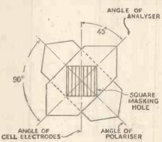
A diagram which shows the relative angle of the nicols and Kerr cell-electrodes. The masking hole and the electrodes are drawn much larger in proportion to the nicols for the sake of clearness
