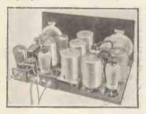
Circuit : six-valve-super-het. Battery version, approximate cost, less valves, £7; A.C. version, approximate cost, less valves, £13 5s.
