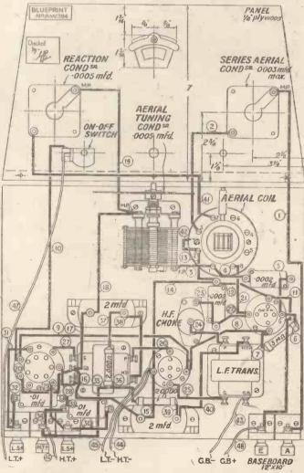
The wiring diagram shown here is a reproduction of the blueprint which has been specially prepared for the "Britain's Favourite Three." Copies of the full-size blueprint can be obtained, price one shilling, post free. Ask for print No. 394
