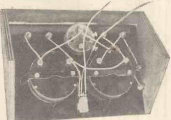
A rear view of the unit wired up so that both meters can be used for testing
