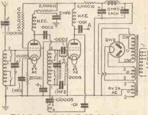
This is the theoretical circuit of the two-stage superhet short-wave converter
