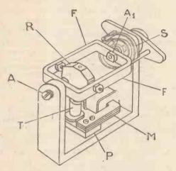
Fig. 2. The oscillating-mirror device patented by Scophony for scanning the line of light produced by the echelon device. The mirror is omitted to show the mechanism more clearly but it is carried in the frame F, its steady swing about the axis of the jewelled bearings A and Al being controlled by the chronometer spring S. A cross-pivoted rocker R limits the swing, and is coupled by shaft T to the armature of a synchronous motor M. P is a platform carrying the stator of the motor
