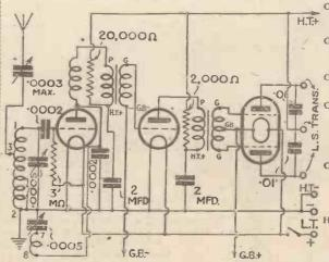
Here's the theoretical circuit diagram of the latest edition of the "Favourite." It has iron-core tuning in place of the previous band-pass arrangement, and class-Boutput. The values of the chief components are indicated
