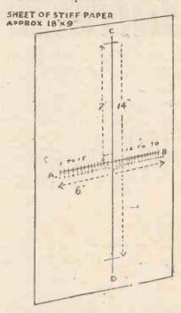
·Here are details of the chart which enables you to adjust the mirror drum
