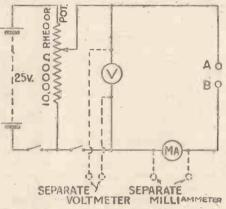
This is a suggested wiring scheme for the tester. The dotted lines show connections which can be made in order to use the meters independently of the resistance testing arrangements
