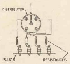
Fig. 2. This diagram shows how the resistances are connected in the ignition circuit
