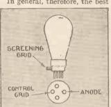
Typical pentode power valve, as used in the output stage for extra power or for economical working. Note that the terminal on the side of the valve base is the screening grid, which is taken to the postive high-tension of the battery, either to the same point as the anode or to a lower voltage
