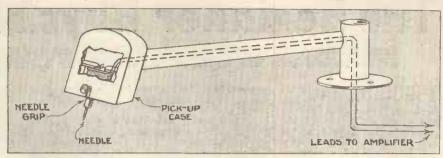
Usually, as here, a pick-up is contained in a small and lightly constructed case fitted to the end of a supporting arm, the leads from the pick-up coil passing through the arm into the base of the arm support
