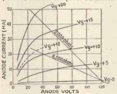
Fig. 1. The anode-current anode-volts characteristics of the 240B valve
