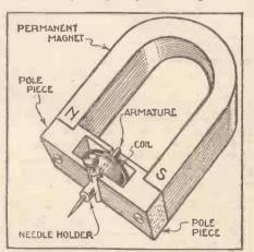
Typical gramophone pick-up construction, showing the coil fitted inside the permanent magnet. The needle vibrations affect the field of the magnet, and as the coil is in this field voltages are set up in the coil, similar to the energy we get from a wireless signal after the detector stage
