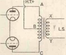
Fig. 2. The output transformer circuit
