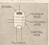
Circuit symbol for a pentode power valve. Note that there are three grids, one of which is inter-nally connected to the filament
