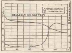
Discharge curves for the Hellesen 99-volt standard capacity battery tested
