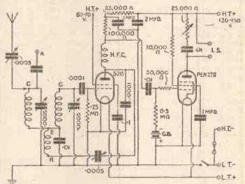
A feature of the circuit is the band-pass aerial tuning and screengrid detector: Note the special resistance-capacity coupling arrangement for the pentode output valve which is tone corrected
