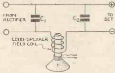
Fig. 6. In some sets the loud-speaker field winding is used as the smoothing choke, thus saving the cost of a special choke. This is done, by the way, in the latest "Home-Lover's" set
