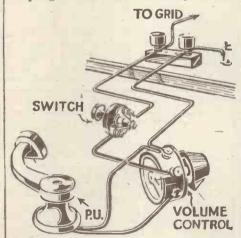
Suitable connections for pick-up, switch and volume control
