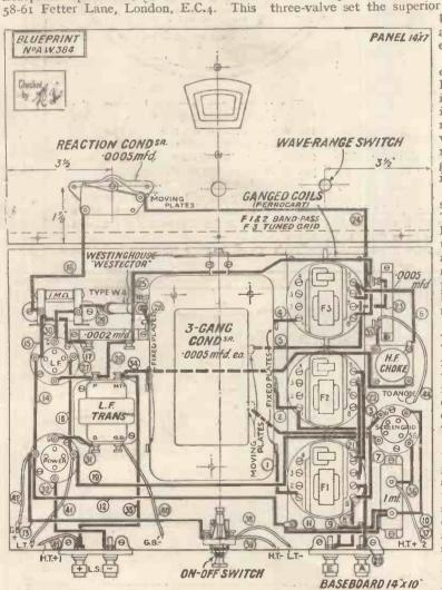
The layout and wiring diagram. It will be noticed that assembly and wiring are quite simple. A full-size blueprint can be supplied, price 1/-
