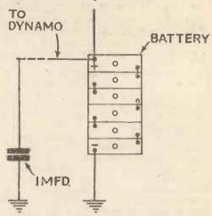
Fig. 3. Condensering the unearthed side of the battery will assist in reducing unwanted noises
