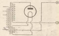
A half-wave rectifier circuit, which needs more smoothing than the full-wave type, but is satisfactory when there is not much low-frequency amplification
