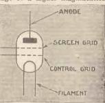
Circuit symbol for a screen-grid valve. You will see that in addition to the normal filament, grid and anode there is a screen-grid
