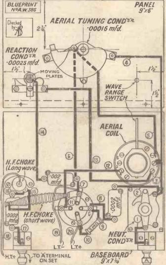
Here is the layout and wiring diagram of the short-wave adaptor.
