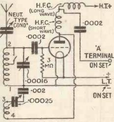
The circuit of the adaptor. A dual range co'l covering 18-32 and 30-64 metres is used but the full switching is not shown
