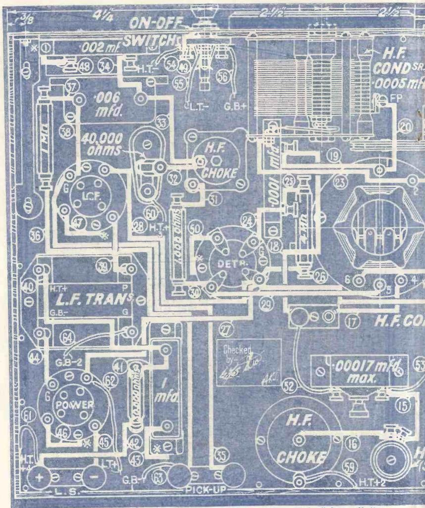
LAYOUT PLAN AND WIRING DIAGRAM OF THE "MELODY RANGER"-"Amateur Wireless," January 28, 1933.
