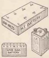
Here are the three batteries needed for operating a wireless set. (Top) A high-tension battery consisting of dry cells in series. (Left) A smaller edition of the high-tension is the grid-bias battery. (Right) The lowtension accumulator, a two-volt cell for heating the valve filaments batteries, and serves as a reminder to replace G.B. batteries periodically.
