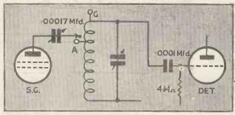
Fig. 4. The selectivity of the intervalve coupling is controllable by means of the pre-set-type coupling condenser between the anode of the screen-grid valve and the tuned-grid circuit of the detector valve
