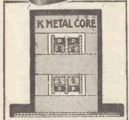
Illustration showing "K" METAL CORE and method of winding as employed in the "Hypermu"
