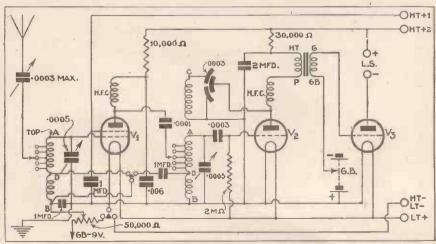
Here is the complete theoretical circuit diagram of the latest version of the "Build As You Learn" screen-grid three-valver. Note specially the modifications in the high-frequency part of the circuit to take the variable-mu type of screen-grid valve
