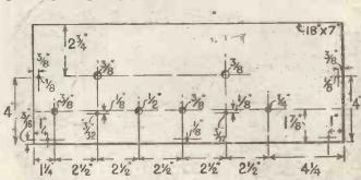
Here is a dimensioned diagram of the panel for use if this is not obtained ready drilled
