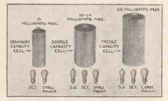
There are three different sizes of high-tension battery for use with wireless sets. This diagram is reproduced to remind beginners that a set taking much more than six milliamperes of anode current cannot be run from the small standard-capacity battery
