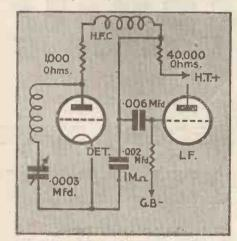
Fig. 5. A 1,000-ohm fixed resistance acts as a short-wave choke in series with the normal high-frequency choke in the anode circuit of the detector. Note the .002-mfd. by-pass condenser connected between the high-frequency choke and low tension
