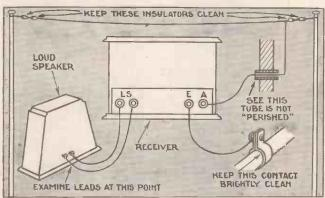
Vulnerable points in the externally-connected accessories of the receiving installation are indicated in this diagram. Watch the aerial system for leakage and inspect the earth for faulty contact every few months. Beware of worn loud-speaker leads—they cause crackles!
