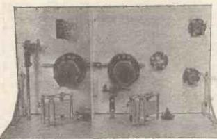
Showing relative positions of coils and valve-holders
