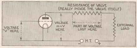
This simple theoretical diagram may help you to understand the action of a valve when it is actually working in the set. Note that the voltage is applied across the grid and filament and appears in an amplified form across the anode and filament
