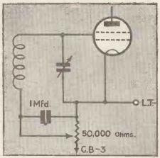
Fig. 2. Volume is controlled by varying the negative grid bias of the variable-mu valve by means of a potentiometer across the grid-bias battery
