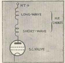
Fig. 3. To provide for efficient reaction on all wavelengths, there is a short-wave choke in series with a long-wave choke in the anode circuit of the screen-grid valve
