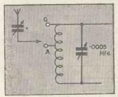
Fig. 1. Aerial coupling is varied by a pre-set condenser connected to alternative tappings on the aerial tuning coil
