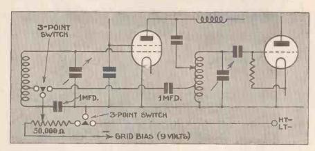
From this detailed circuit diagram of the high-frequency and detector portions of the screengrid three-valver you should be able to understand how the three-point switch is used to cut out the grid-bias battery when the set is not in action. Note carefully the 1-microfarad fixed condenser between one point on the three-point switch and the wave-change switch point of the detector grid coil
