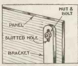
used. If there is any inaccuracy in the drilling you can correct for this simply by sliding the bracket along a little, the U-shaped holes enabling this to be
