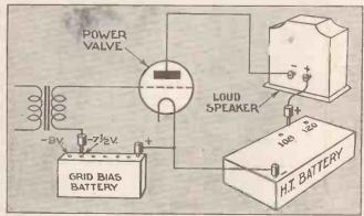
The heart of your set is the valve of each stage. Here you see how a valve gets its anode voltage from a high-tension battery and its gridbias voltage, which is intimately connected with the high-tension supply, from a smaller battery called the grid-bias battery. When the positive voltage of the high tension drops with battery age you must remember to reduce the negative bias on the grid
