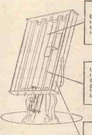
Extremely close spacing of the electrodes, assuring high slope.
