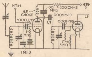
Fig. 1. A good short-wave circuit in which a screen-grid valve is used
