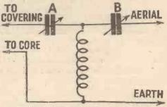
Fig. 2. A filter circuit which is put between the sheathed aerial and the set. A is the tuning condenser and B the coupler
