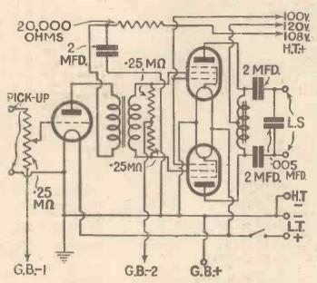
Although this amplifier has pentodes in push-pull, the circuit is quite simple. The input transformer has quarter-megohm leaks across the secondary, to avoid the necessity for a special tapped secondary transformer, and the output is taken through a choke and double condenser arrangement, so that no tapped output transformer is needed. These are factors which make the amplifier cheap to build
