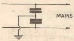
Fig. 1. A simple filter circuit to by-pass H.F. interference on electric light wires. The centre connection between the two condensers is earthed
