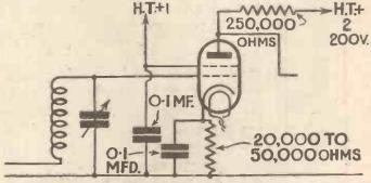
the MS4B operates well as a detector under its normal amplifying conditions.
