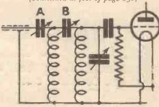
Fig. 3. A complete circuit using the sheathed aerial and the filter shown by Fig. 2
