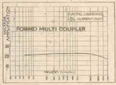
This curve shows the effective amplification of the Formo Multi-coupler plotted against frequency
