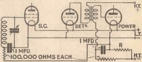
This is a typical three-valve circuit in which automatic blas is applied by means of voltage-dropping resistances
