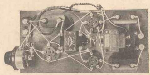
This plan view shows the simple construction of the amplifier, with all the components mounted on a baseboard
