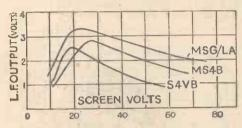
Fig. 5. The optimum screen voltage is more critical with the anode-bend-circuit and is also distinctly lower
