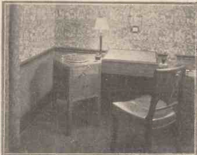
One of the new gramophone broadcast consoles of the type used at Savoy Hill
