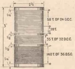
Fig. 3. Winding data for dual-range coil
