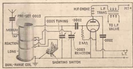
Fig. 4 .Suggested circuit for using dual-range coil
