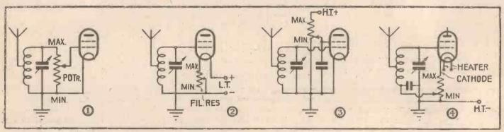
Fig. 1. Input volume control. Fig. 2. Filament resistance volume control. Fig. 3. Screen-grid type volume control. Fig. 4. Grid bias control of A.C. mains screen-grid valve
