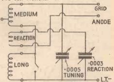
Fig. 2. Dual-range coil with reaction winding
