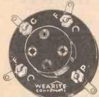
Suitable for use in the "Century Super Portable." This valve holder is fitted with sockets which are split in four places and are therefore ideal for the new solid pins fitted to modern valves.
