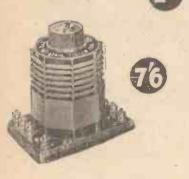
THE TELSEN AERIAL COIL.—The latest development in Dual Range Aerial Coil Design. Incorporates a variable series condenser which can be set to give any degree of selectivity, making coil suitable for ALL districts. This adjustment also acts as an excellent volume control. The waveband change is effected by means of a three-point switch. A reaction winding is included. Price 7/6 each.
