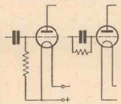
Two ways of connecting the grid leakfrom grid to filament and directly across the grid condenser
