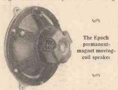
coil itself which is smaller than usual, being just under I inch in diameter, is mounted on a machine-made paper diaphragm, which in turn is suspended from a leather surround. The whole assembly is mounted on a rigid metal chassis arranged for screw or bolt fixing to the baffle board or cabinet in which it is to be mounted.
