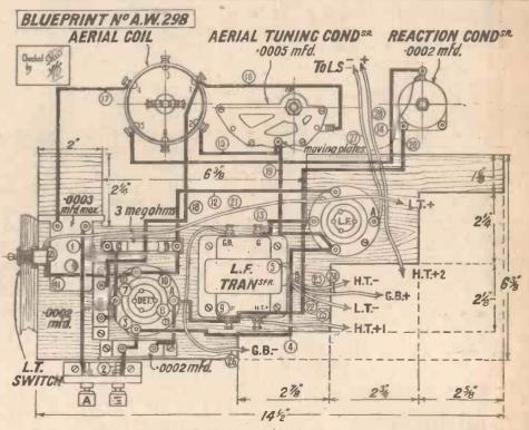
The layout and wiring diagram of the actual receiver. A full-size blueprint is available, price 1/-
