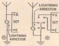
How a lightning arrestor is installed. Fig. 2b. Arrangement of lightning arrestor and earthing switch
