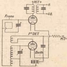
Fig. 3. Connections of first detector and oscillator
