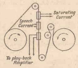
Schematic design showing the principle of the Blattnerphone talking-tape machine
