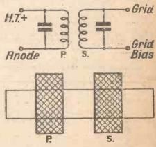
Fig. 2. Band-filter coil for super-het
