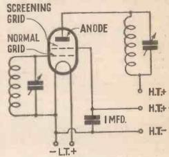
Fig. 2. Connections of screen-grid valve in tuned-anode circuit
