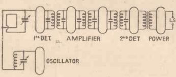
Fig. 1. Arrangement of valves in super-het receiver
