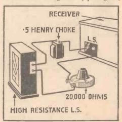
Fig. 3. Simple low-note suppressor circuit
