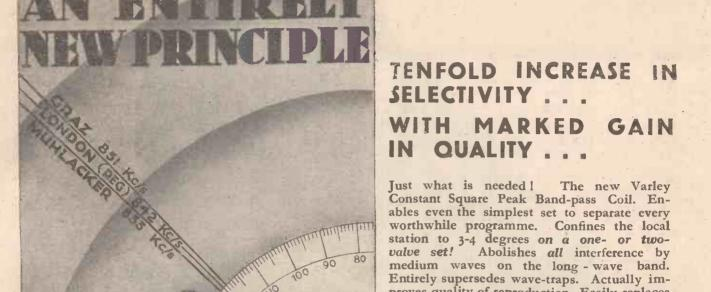
The new Varley Constant Square Peak Coil (Regd. Design No. 763904. Prov. Pat. No. 2485/31) gives a constant squared-topped peak separation of substantially nine kilocycles on the whole of the medium and long wave range. It covers both wavebands, and is supplied complete with extension handle for switch and a bracket for horizontal or vertical mounting.
