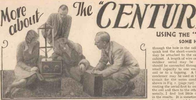
THE third position of the oscillator switch, as I pointed out last week, is for short waves, from about metres. Thus the switch has three positions, short, medium and long, and so far we have dealt only with the medium and long wavelengths. This is because the frame aerial used is suitable only for these wavelength ranges.
