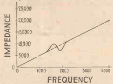
Fig. 1. Typical impedance curve for a cone speaker
