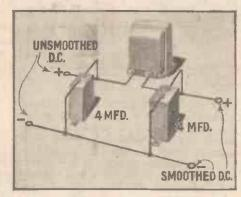
The essentials of a filter are condensers and choke as shown pictorially above
