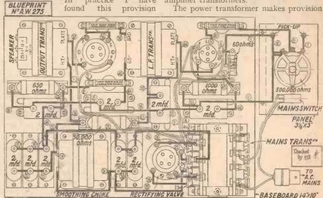
The layout and wiring diagram, of which a full-size blueprint is available, price 1/-
