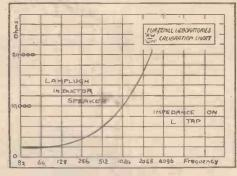
Characteristic curve of the new Lamplugh inductor speaker
