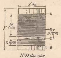
The coil can very easily be made at home, all the necessary details being given by this drawing
