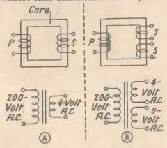
Fig. 1. Simple transformer connections
