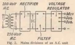
at the input voltage suggested the current would be .06 ampere.
