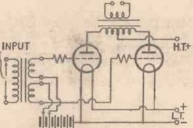
It is usually advisable to have separate grid bias for each valve of a push-pull combination, and this circuit shows how a split-secondary transformer enables separate bias values to be applied
