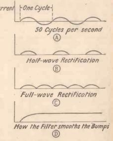
Fig. 3. How the A.C. is converted into D.C.
