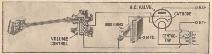
This pictorial diagram shows how "automatic" grid bias can be applied to the first A.C. valve in a gramophone amplifier. Note the volume control between this valve and the pick-up
