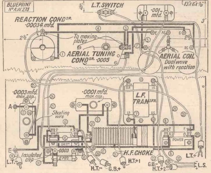
An enlarged drawing of the wiring showing the connections between the components mounted in the case and those on the backboard
