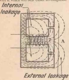
Fig. 1. Magnetic system of moving-coil speaker showing disposition of the flux
