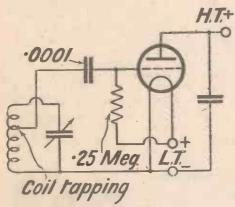
Fig. 4. The tapped coil shown here overcomes the loss incurred by grid-leak damping
