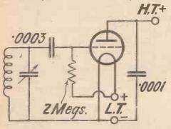
Fig. 1. Normal arrangement and values for leaky-grid-condenser detection
