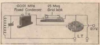
Fig. 2. For power-grid detection low values of grid leak and condenser must be used
