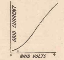
Note how the grid current increases as the grid voltage is increased
