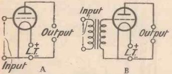
Fig. 1 (A). A skeleton valve amplifying circuit. (B) Transformer coupling arrangement for L.F. valve
