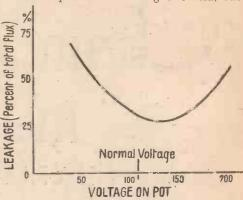
Fig. 2. Curve showing field strengths at different voltages
