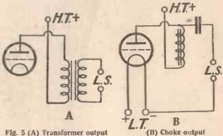
Fig. 5 (A) Transformer output
