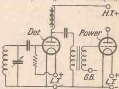
Fig. 5. In this circuit the anode current is diverted from the transformer primary to a special choke
