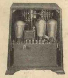
The back of the Ediswan Power Pentode Two: note the special coils at the top
