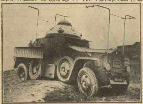
Another radio aid for the Army. Following on the news of the radio-equipped tanks comes this eight-wheeled armoured car, which is fitted up with a transmitter and a receiver, so that it can keep in touch with its objective while on the move. This new monster—a Crossley—is having its eight-wheel chassis and its radio gear tested out in the Derbyshire hills
