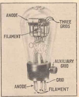
The pentode valve is of somewhat different construction, to the ordinary valve: note the extra terminal
