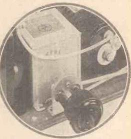
"On no account make twisted loose connections to the mains point, but employ a proper recessedcontact plug and socket"
