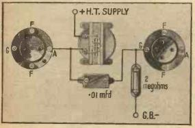
Fig. 2. The choke-capacity method does not give a voltage step-up
