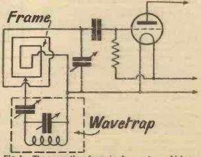
Fig. 1.—The connections for a simple wavetrap which can be added to most transportable sets. It is described in the accompanying article
