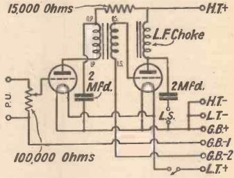
Here is the circuit; note the volume control and choke output
