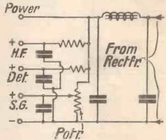
Fig. 2. Voltage regulating and smoothing circuit of mains unit
