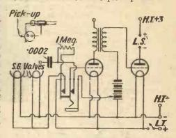
Circuit of battery-operated set showing pick-up connections
