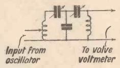
Fig. 3. Capacity-coupled filter circuit
