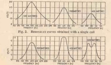
Fig. 4. Curves obtained with a capacity-coupled filter
