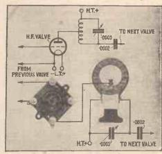
Fig. 2. The tuned-anode coupling is the simplest
