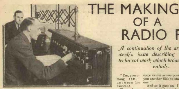
The picture shows the Dramatic Control Panel by means of which the productions of several studios are blended before being actually transmitted
