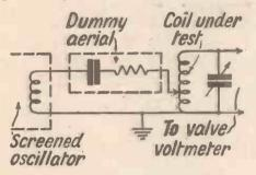
Fig. 1. The circuit used for test
