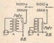
Fig. 4. Another system of connections for a volume control
