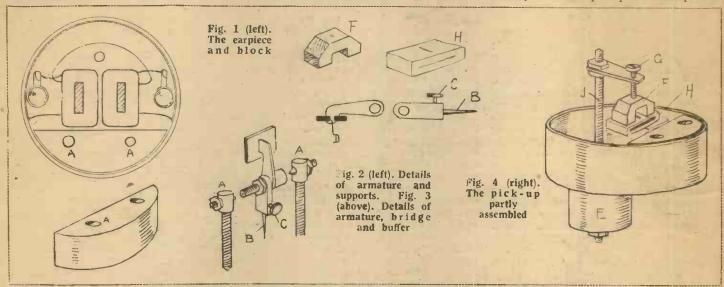
You will need nothing but a single earpiece from a pair of headphones, three contact studs, some small pieces of wood, brass and iron, a piece of rubber sponge, and a few odd screws and nuts.
