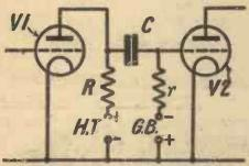
Fig. 1. Diagram of resistance-coupling system
