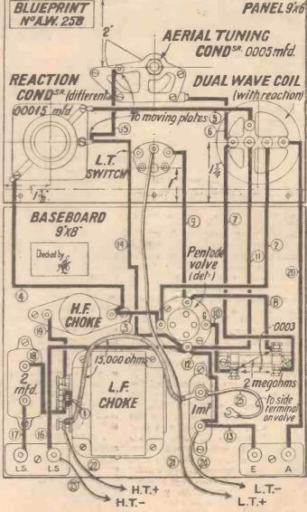
Here is the layout and wiring diagram. A plan view which will be helpful appears on the next page
