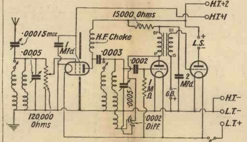
The circuit of the "Challenge Three." Features are the novel volume control which does not affect tone or tuning, differential reaction and efficient L.F. filtering
