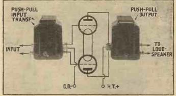
Fig. 2. Here is a better system with valves connected in push-pull, which allows of using a lower H.T. voltage
