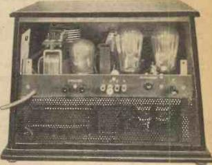
The internal arrangements of the Varley Junior Two are particularly neat: note the accessibility of the valves particularly neat: and the efficient disposition of the mains apparatus
