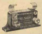
TELSEN FIXED (MICA) CONDENSERS. Shrouded in genuine Bakelite, made in capacities up to .002 mf. Pro. Pat. No. 20287/30. .0003 supplied complete with Patent Grid Leak Clips to facilitate series or parallel connection. Can be mounted upright or flat. Tested on 500 volts.
