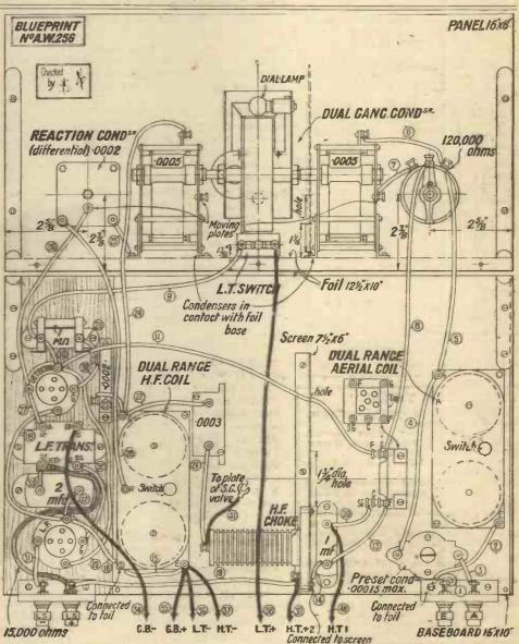
The wiring diagram. A full-size blueprint, which is a great help in constructing, can be obtained, price 1/-
