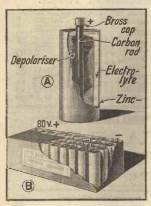
This picture shows the features of a dry cell and the assembly of a H.T. battery
