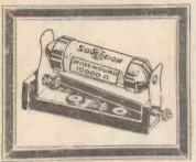
Illustration shows Sovereign Wire Wound Resistance with Bakelite holder and metal supports and terminals.
