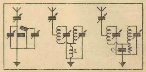
Fig. 3. An early double-tuner arrangement. Fig. 4. A coupled circuit with magnetic coupling. Fig. 5. A coupled circuit with condenser coupling
