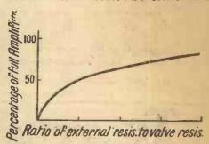
Fig. 2. Curve showing amplification obtained from a valve in terms of anode resistance
