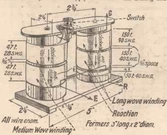
The particulars given in this drawing are sufficient to enable constructors to build the coils
