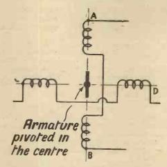
This diagram shows the principle upon which the induction motor works
