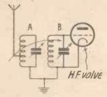
Fig. 2. A coupled aerial-grid circuit
