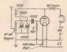
One-valve reaction circuit with potentiometer grid-leak connection
