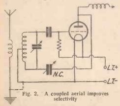
copper foil between the panel and the condenser itself. Care must, of course, be taken to see that the foil which is connected to L.T.— does not touch any metal parts on the condenser itself, as otherwise a short-circuit will result. The aerial is coupled through a small condenser (which may be either a .ooor fixed condenser or a pre-set condenser) on to the grid end of the coil, while the earth connection is taken to L.T.—, as shown in the figure. Such a circuit will be found to
