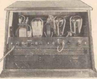
The accessibility of the receiving valves and valve rectifier is clearly shown in this view of the back of the Varley All-electric Two-valve set.
