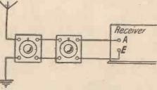
Diagram showing how two by-pass units may be used at the same time
