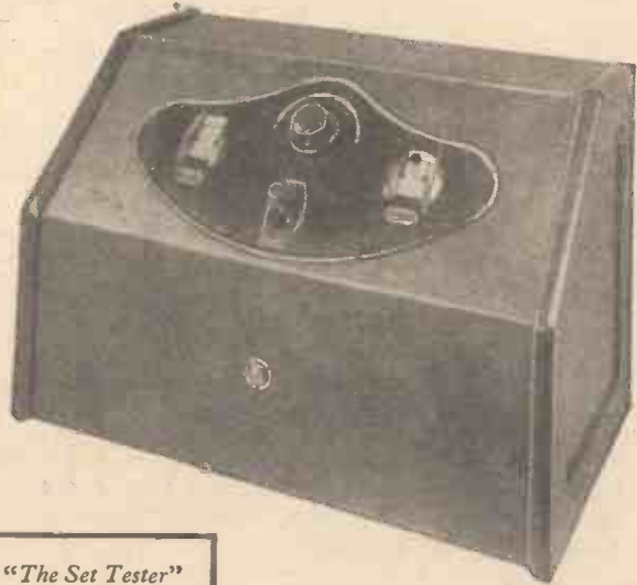
The fabric-covered metal case of the Ediswan receiver is an innovation
